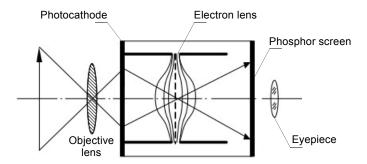
Fig. 1. Structure chart of image intensifier system.
