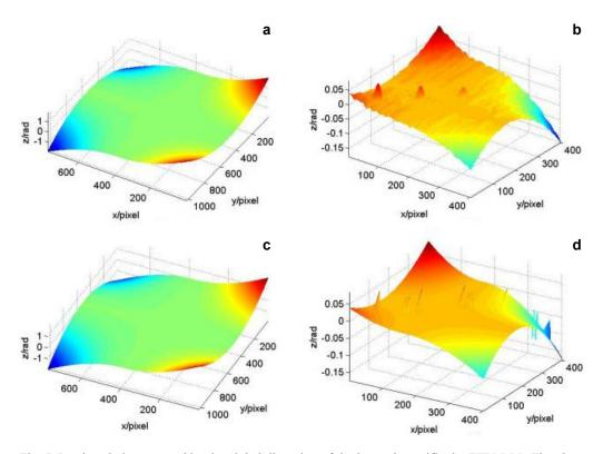
Fig. 7. Retrieved phase caused by the global distortion of the image intensifier by FTPM (a). The phase distribution caused by partial distortion extracted from image  $\mathbf{a}$  (b). Retrieved phase caused by the global distortion of the image intensifier by PPSG (c). The phase distribution caused by partial distortion extracted from image  $\mathbf{c}$  (d).
