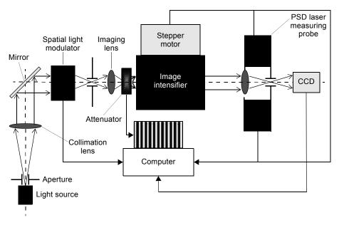
Fig. 3. Schematic of measuring system.
