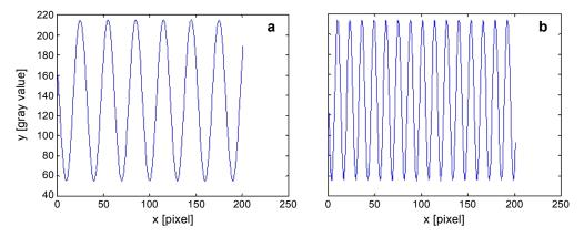
Fig. 5. The fidelity of sinusoid of designed grating. The sinusoid at a line when  $T_0 = 30$  pixels (a) and at the same line when  $T_0 = 13$  pixels (b).
