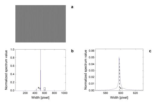
Fig. 4. Processing of captured grating. The captured grating (a). The normalized spectrum of the captured grating a (b). The extracted fundamental frequency from the spectrum b (c).
