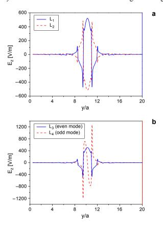
Fig. 4. The  $E_z$  fields along lines  $L_1$  and  $L_2$  in Fig. 3a (a). The  $E_z$  fields along lines  $L_3$  and  $L_4$  in Fig. 3e (b).
