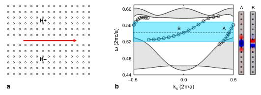
Fig. 1. The UAW structure model (a) and the project bands of the coupled modes (b). The dashed line denotes  $\omega = 0.542 (2\pi c/a)$  that interacts with the two curves at points A and B, and the corresponding eigenfields of A and B are also shown. The project wave vector  $k_x$  is along the waveguide direction.
