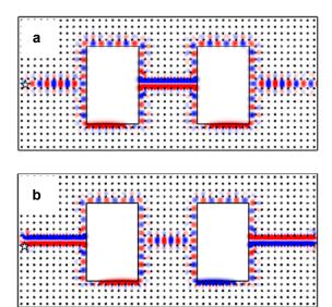
Fig. 5. Continuous mode transformations. Even mode to odd mode to even mode (a). Odd mode to even mode to odd mode (b). The five-pointed star denotes the position of a source.
