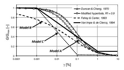
Fig. 4. Comparison of some models of soil modulus degradation
