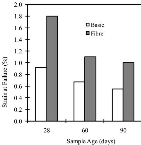
Fig. 7. Strains at failure achieved for samples tested at cell pressure of 60 kPa (undrained triaxial test condition)
