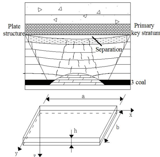
Fig. 2. Schematic diagram of the plate structure
