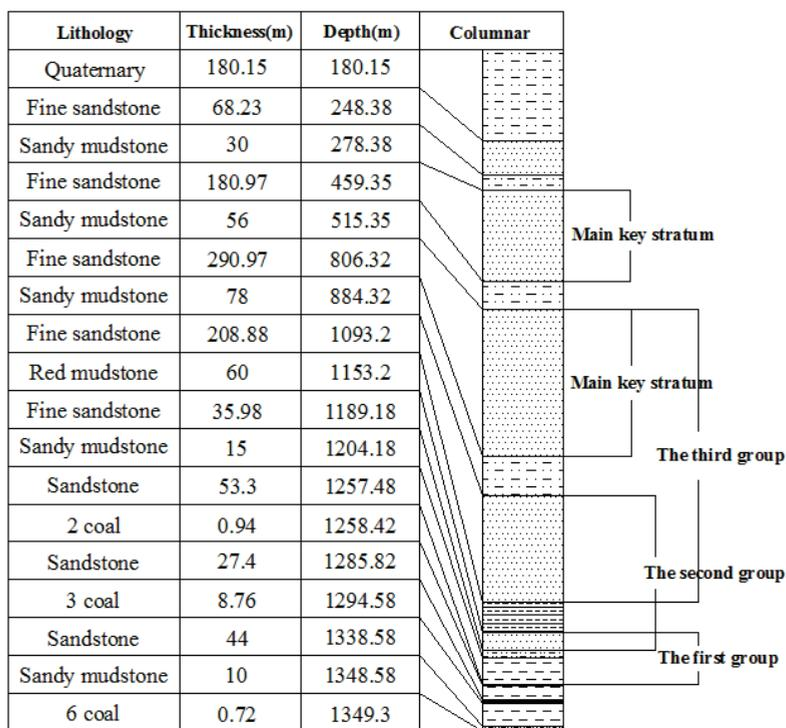
Fig. 1. Column diagram of No. 3 coal in Gucheng Coal Mine
