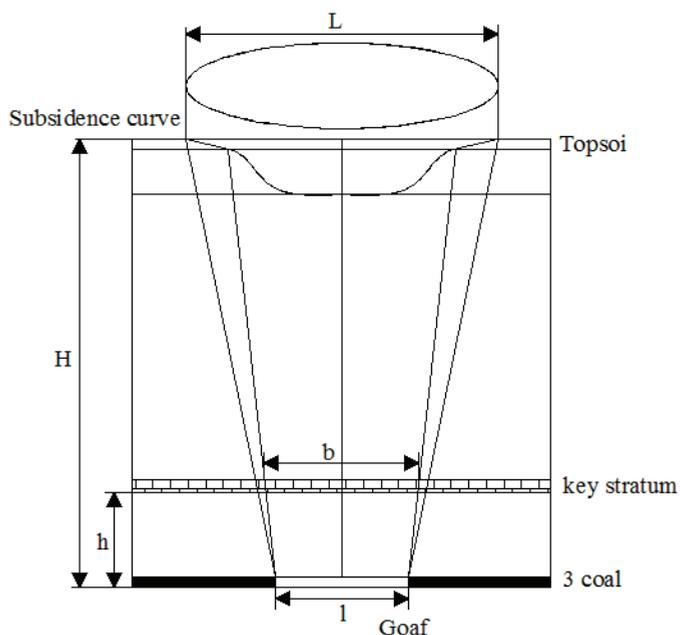
Fig. 3. Schematic diagram of rock movement
