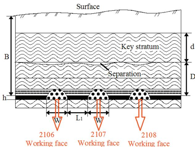
Fig. 5. Key stratum large-scale separation mechanics model
