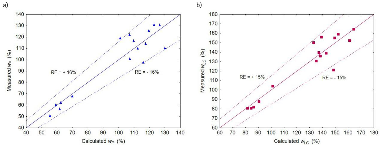
**Figure 6:** Comparison between the measured and calculated values: a)  $w_p$  and  $w_p$  from Equation (30) in Table 5, b)  $w_{LC}$  and  $w_{LC}$  from Equation (33) in Table 5 of Eemian gyttja, with zones of maximum RE for regression models.
