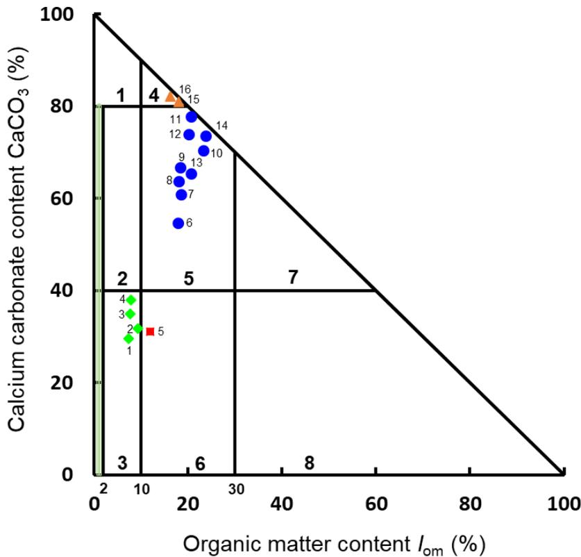
**Figure 1:** Tested samples of Eemian gyttja according to the classification of Długaszek [7]:  $I_{om} = 0\%–2\%$  mineral soils. Note: 1, low organic lacustrine marl; 2, high calcareous mineral gyttja; 3, low calcareous mineral gyttja; 4, high organic lacustrine marl; 5, high calcareous mineral-organic gyttja; 6, low calcareous mineral-organic gyttja; 7, high calcareous organic gyttja; 8, low calcareous organic gyttja; ◆●▲ 1–16, test number
