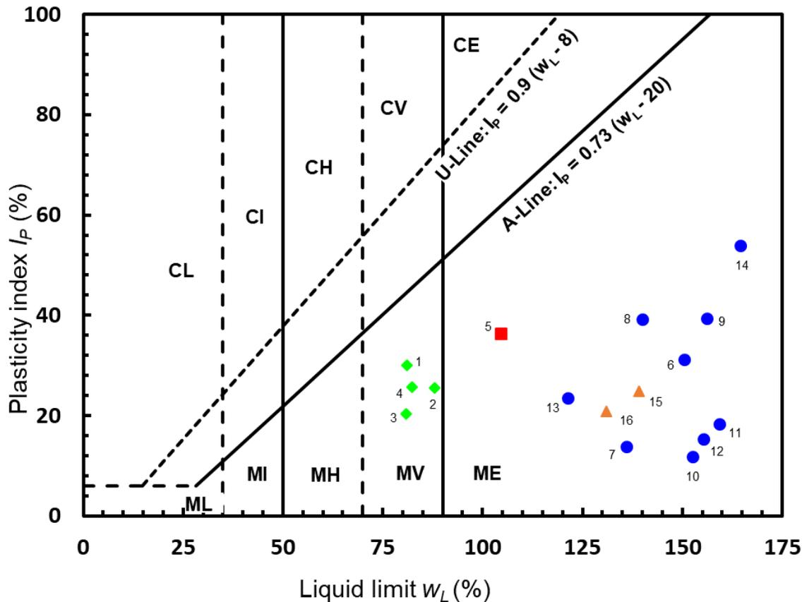
**Figure 2:** Tested samples shown on Casagrande's plasticity chart.
