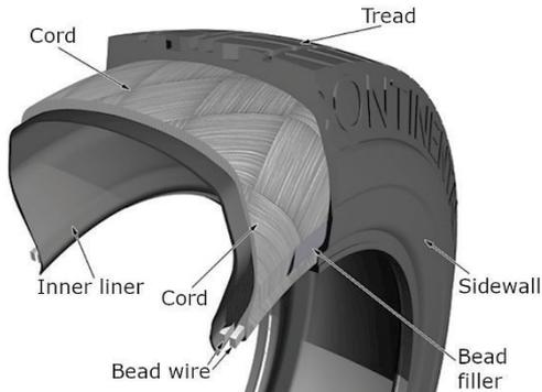
**Fig. 1.** Construction of the diagonal tire
