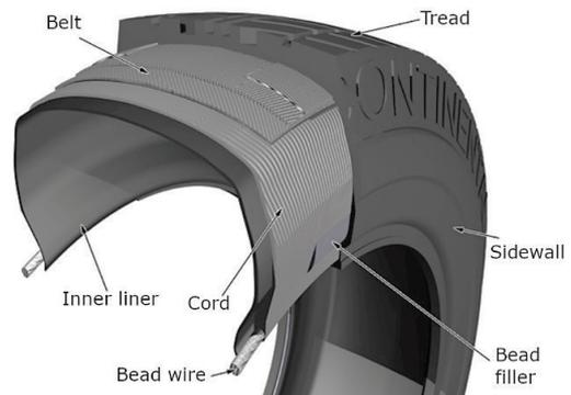
**Fig. 2.** Construction of the radial tire
