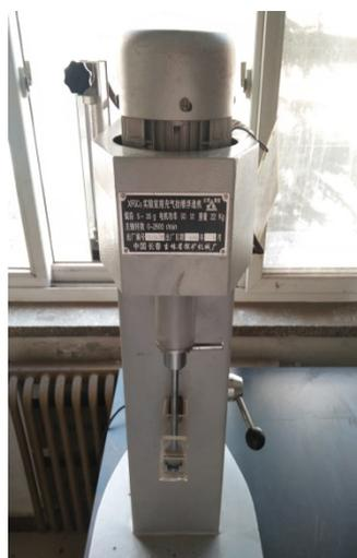
Fig. 2. XFG flotation machine for micro flotation tests
