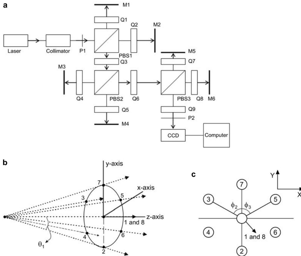
Fig. 1. Experimental setup for generation of hexagonal arrays, P – polarizers, PBS – polarizing cube beam splitters, Q – quarter-wave plates, CCD – charged coupled device – a; Schematic of the path of all eight beams – b; Location of the center of eight beams in the transverse plane, defining  $\phi_p$  – c.
