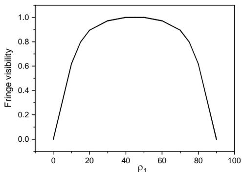
Fig. 4. Fringe visibility curve for the orientation of the quarter-wave plate Q9.
