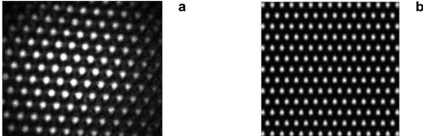
Fig. 2. Hexagonal array pattern at the out put of third stage of interferometer (a) recorded onto CCD, (b) computed pattern.
