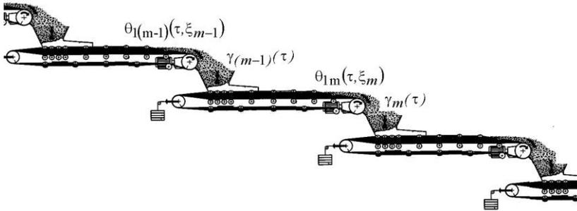
Fig. 2. The scheme of the multi-conveyor system
