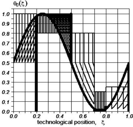
Fig. 5. The linear density of the rock along the route at times  $\tau = 0.025i, i = 1 \dots 23, a = 0$
