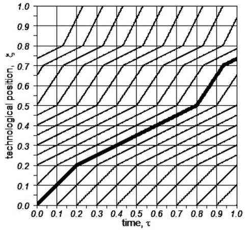
Fig. 4. The motion trajectories for a single material element located in different conveyors of the transport route
