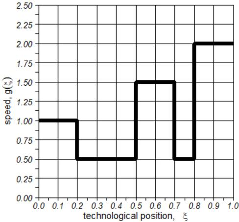
Fig. 3. The belt speed of the long distance transport system depending on the conveyor
