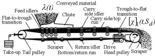
Fig. 1. Schematic diagram of the conveyor
