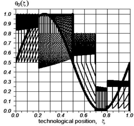
Fig. 6. The linear density of the rock along the route at times  $\tau = 0.025i, i = 1 \dots 23, a = 0,25$
