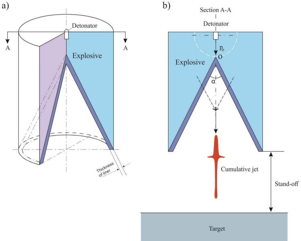
Fig. 1. Scheme of a conical shaped charge (CSC)
