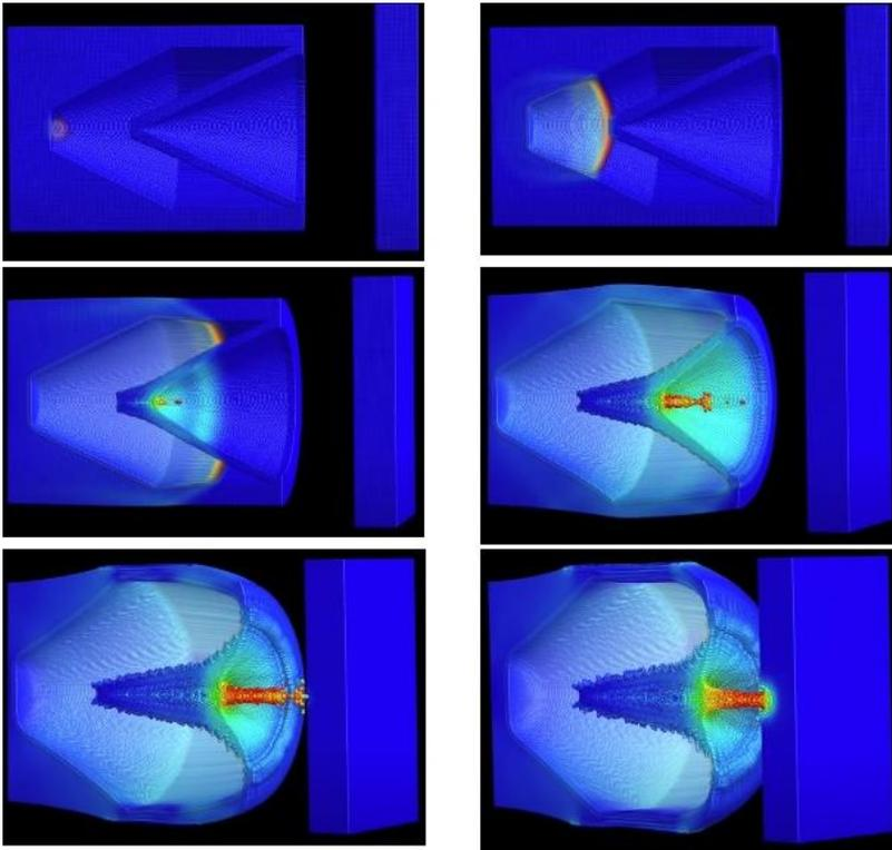
Fig. 2. Successive stages of formation of the cumulative jet
