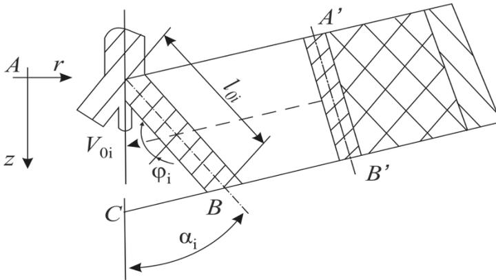
Fig. 4. Scheme of the formation of elements of a cumulative knife
