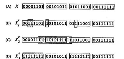
Figure 2.1. Three types of u-errors: Sample codeword (A); 4-unidirectional  $0 \rightarrow 1$  error (i.e. t=4) (B); Burst unidirectional  $0 \rightarrow 1$  error (i.e. b=11) (C); 2-byte unidirectional  $0 \rightarrow 1$  error (in bytes  $B_1$  and  $B_3$ ) (D)
