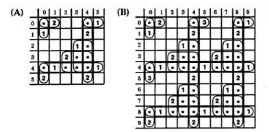
Figure 6.5. Modification map of the AND gates p(j,k) in the STCs for the Borden codes:  $C(n,3), n \in \{8,9,10\}$  (A); C(18,3) (B)
