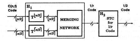
Figure 6.1. The new STC for Borden code C(n,t)
