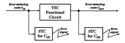
Figure 1.1. General scheme of the self-checking system
