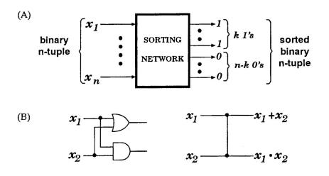
Figure 4.4. The structure of an SN considered here (A); Logic gate implementation of a comparator cell (B)
