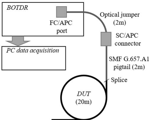
Fig. 1. Measurement system block scheme.
