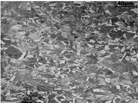
Fig. 3. Structure of 27Mn-4Si-2Al steel solution heat-treated from a temperature of 900 °C after deformation with reduction 20%
