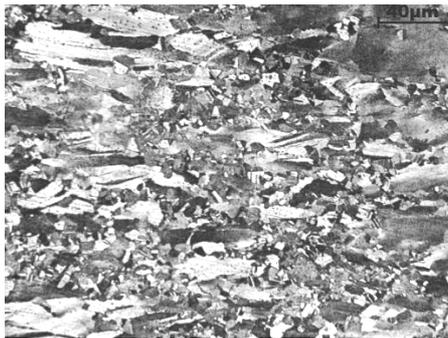
Fig. 6. Refined structure of 27Mn-4Si-2Al steel solution heat-treated from a temperature of 1000 °C after deformation with reduction 40%
