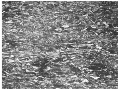
Fig. 4. Refined structure of 27Mn-4Si-2Al steel solution heat-treated from a temperature of 900 °C after deformation with reduction 40%
