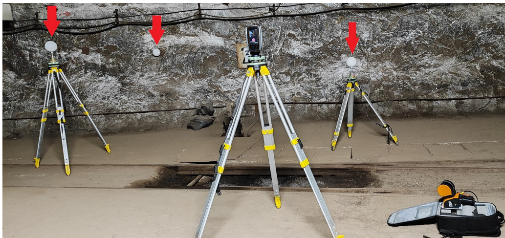
Figure 2: Measurement site with a laser scanner in a mining excavation. A stationary scanner is visible in the central part of the photo. In the lower right corner, there is a mobile scanner intended to perform the measurement. In the background, three measuring spheres are marked with red arrows – two spheres placed on tripods under the geodetic network points and one additional sphere attached to the side of the excavation.
