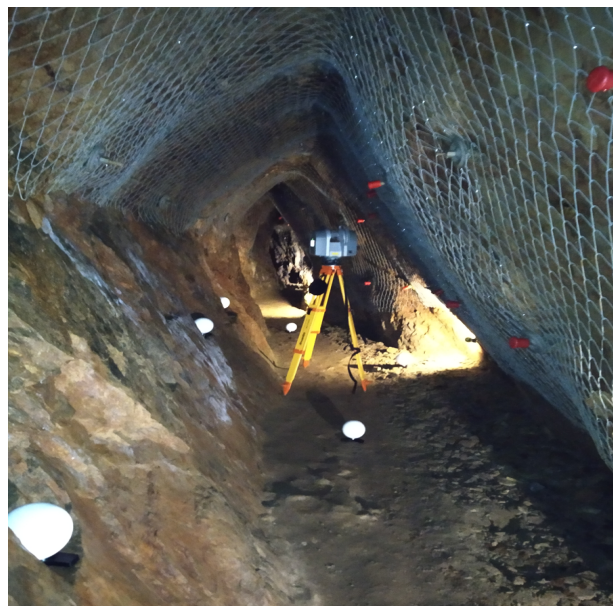
Figure 2: Trimble TX8 laser scanner during measurements in the St. John Adit.
