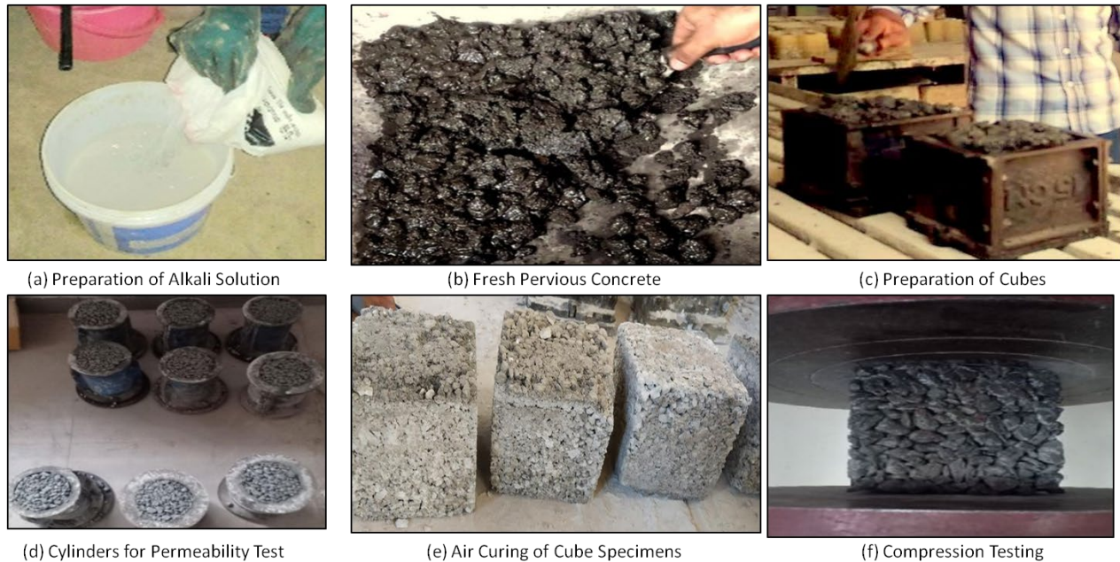
Figure 3: Preparation, air-curing, and testing sequence of geopolymer pervious concrete specimens.
