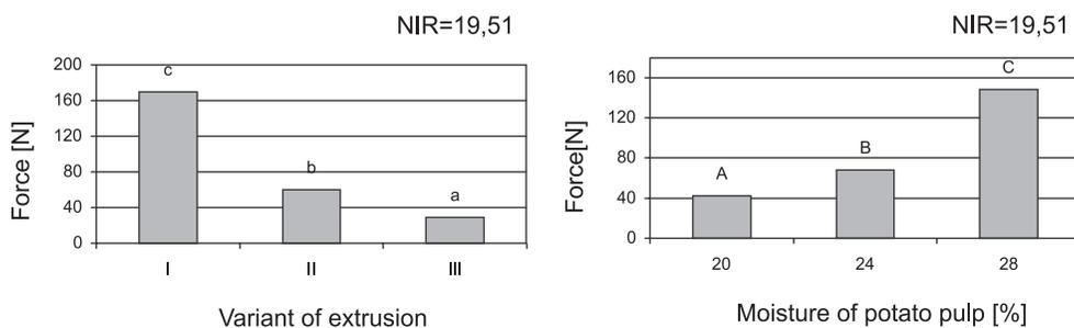
Fig. 2. Influence of extrusion temperature and moisture of potato pulp on maximum force needed for intersection of extrudates
