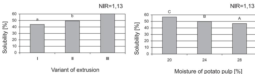
Fig. 5. Influence of extrusion temperature and moisture of potato pulp on solubility of obtained extrudates
