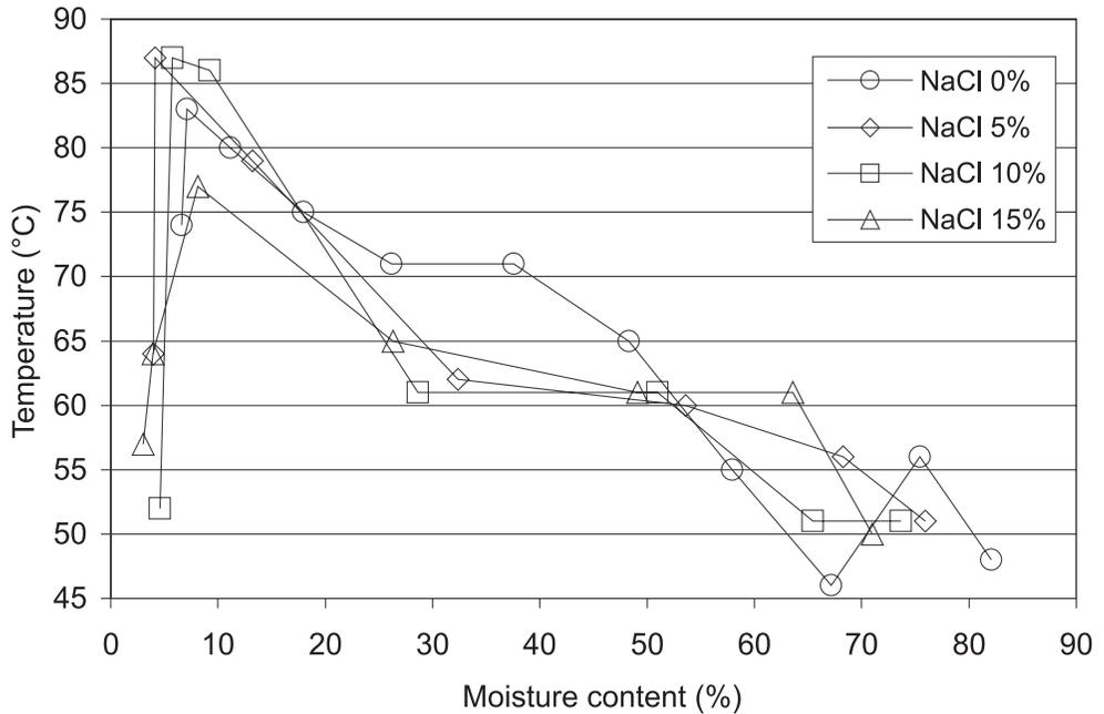
Fig. 4. Temperature profile for pumpkin slices during VM finish drying after pre-drying in different concentrations of NaCl solution
