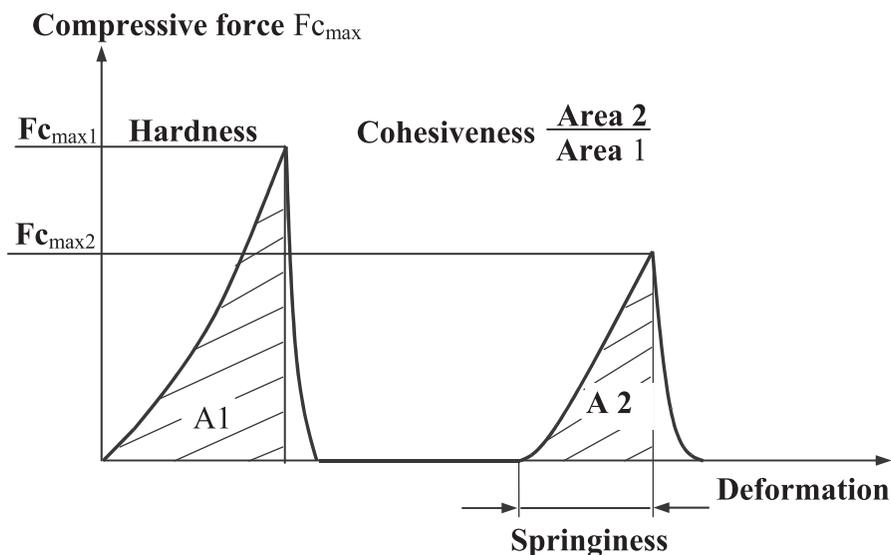
Fig. 1. TPA curve.  $F_{c_{max1}}$  – maximum compressive force at first compression,  $F_{c_{max2}}$  – maximum compressive force at second compression,  $A1$  – force area during the first compression,  $A2$  – force area during the second compression
