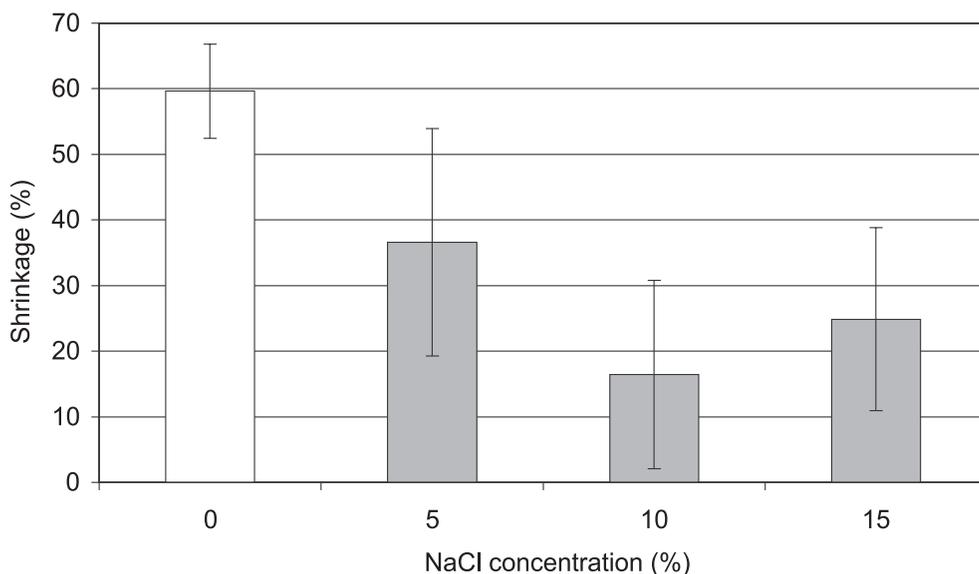
Fig. 5. Effect of NaCl concentration on shrinkage of VM finish dried pumpkin slices
