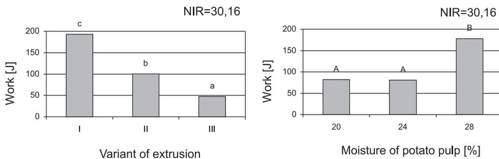
Fig. 4. Influence of extrusion temperature and moisture of potato pulp on work needed for intersection of extrudates
