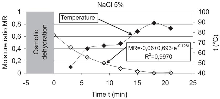
Fig. 3. VM drying kinetics of beetroot slices pre-dried in NaCl solution of concentration 5%
