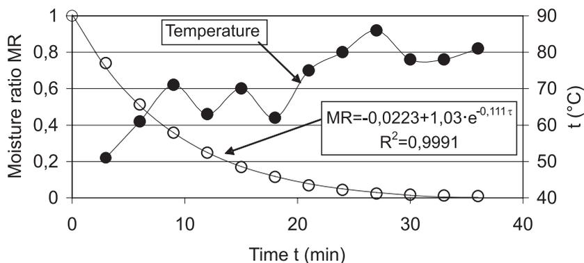
Fig. 2. VM drying kinetics of beetroot slices without pre-drying in NaCl solution
