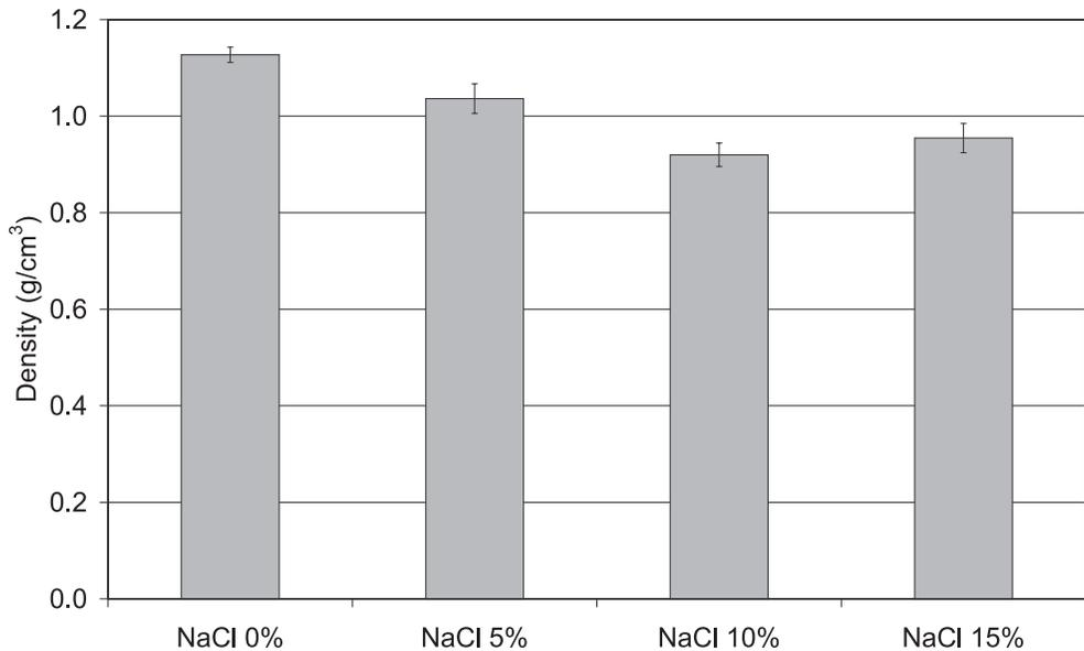
Fig. 6. Effect of NaCl concentration on density of VM finish dried beetroot slices
