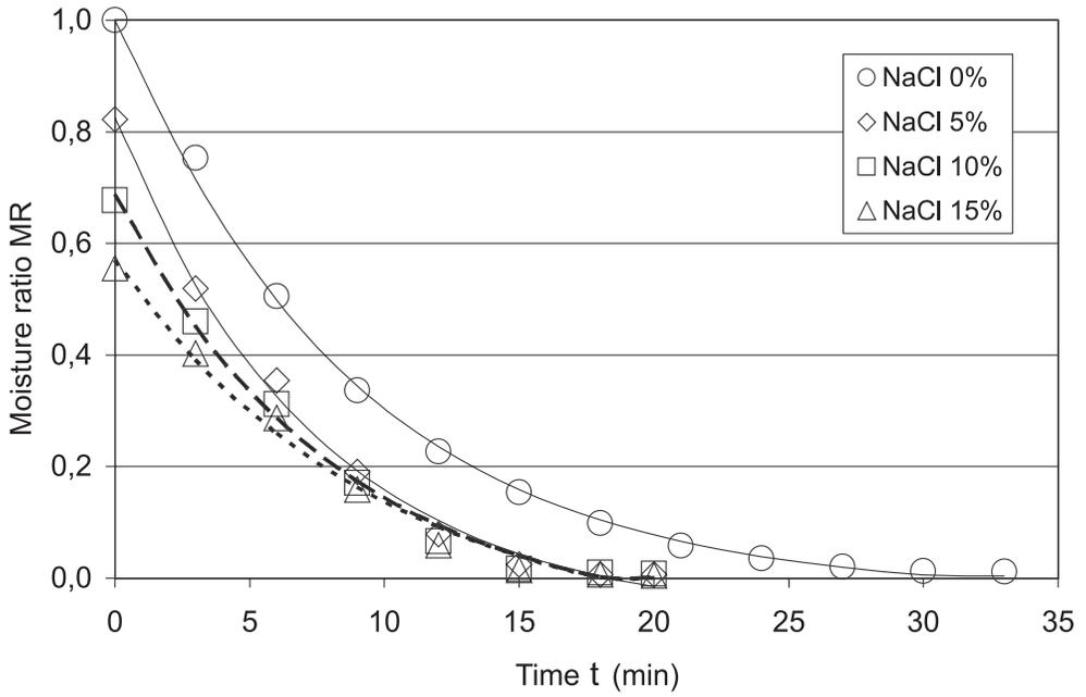
Fig. 3. VM drying kinetics of pumpkin slices pre-dried in different concentrations of NaCl solution
