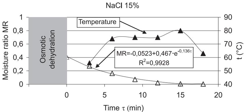
Fig. 5. VM drying kinetics of beetroot slices pre-dried in NaCl solution of concentration 15%
