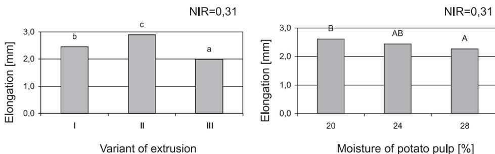
Fig. 3. Influence of extrusion temperature and moisture of potato pulp on elongation causing maximal stress needed for intersection of extrudates
