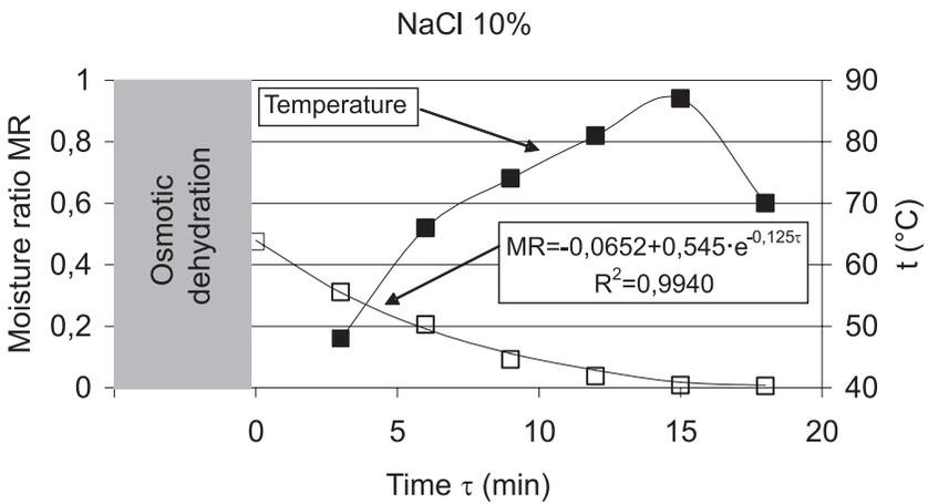
Fig. 4. VM drying kinetics of beetroot slices pre-dried in NaCl solution of concentration 10%
