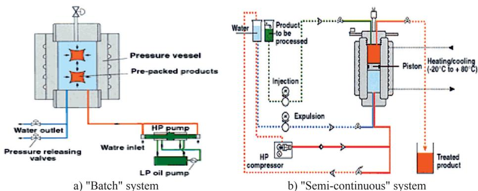
Fig. 1. Patterns of high pressure processing devices designed for food preservation [28,30,37]
