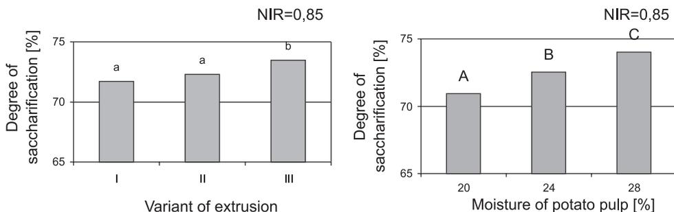
Fig. 7. Influence of extrusion temperature and moisture of potato pulp on degree of saccharification of obtained extrudates
