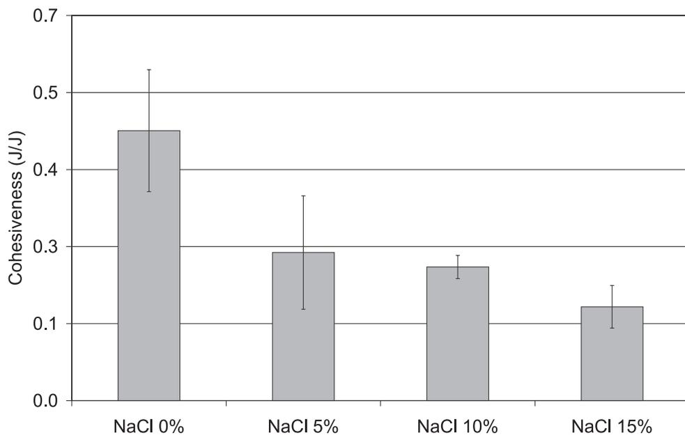
Fig. 10. Effect of NaCl concentration on cohesiveness of VM finish dried beetroot slices
