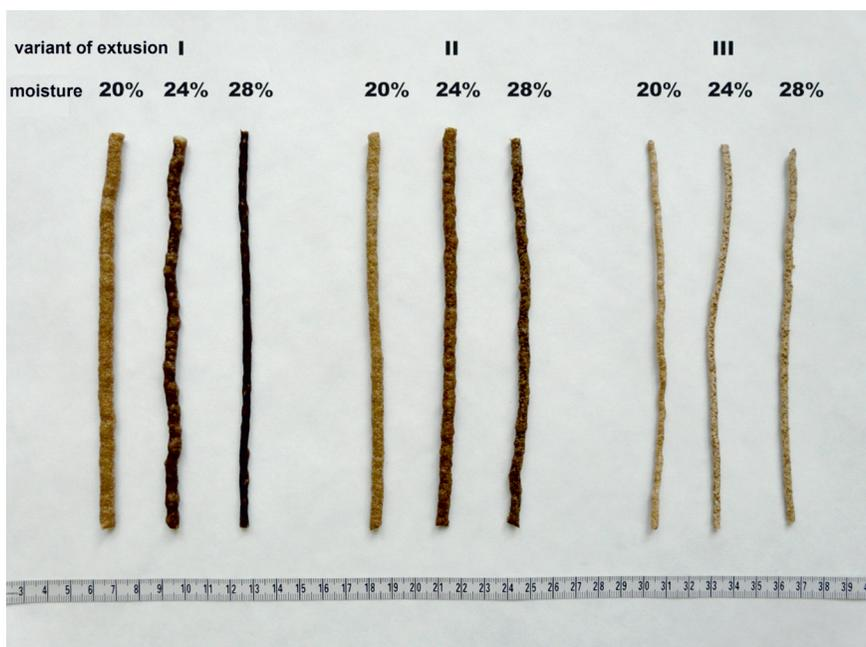
Fig. 1. Appearance of preparations obtained from diverse variants of temperature, and different moisture of potato pulp
