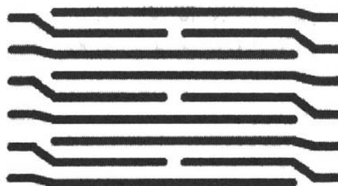
Fig. 16.4. Structure of belt splice.
