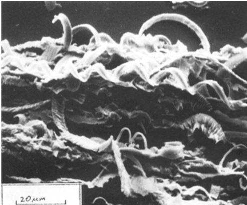
Fig. 10.8. Sheared products of wear of mating surfaces [10.15].
