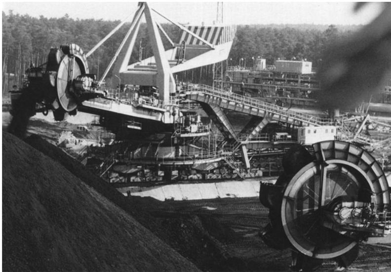
Fig. 17.4. View of LZKS loader-stacker.
