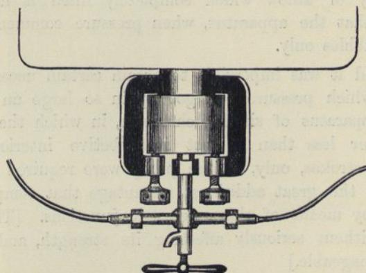
tightly-fitting steel plug which was forced into the upper end of the cylinder after the thermometers and other apparatus had been inserted, and the whole had been filled with water. The plug was forced down by the weight of an assistant standing on it, while a stop-cock at the bottom of the cylinder was kept open for the escape of water, until a massive steel key could be put in through a slot in the side of the cylinder to lock the plug in its definite position.
