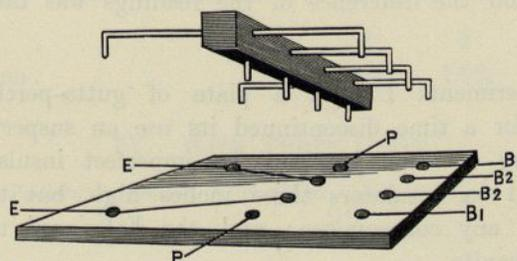
quadrants of the electrometer, *P* with the electrodes, *B*<sub>1</sub> with the decomposing battery, and *B*<sub>2</sub> with the auxiliary (or charging) battery. Also metallic connection, as indicated in the sketch, is permanently established between the two central holes and the holes connected with the electrometer.
