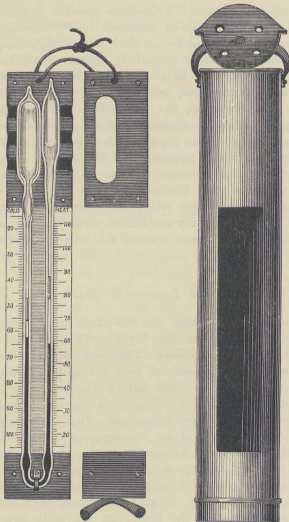
first invented form of protected thermometer, which (so far as I know) was introduced by Sir William Thomson<sup>1</sup>, is simply that the bulb only is protected, the stem being
