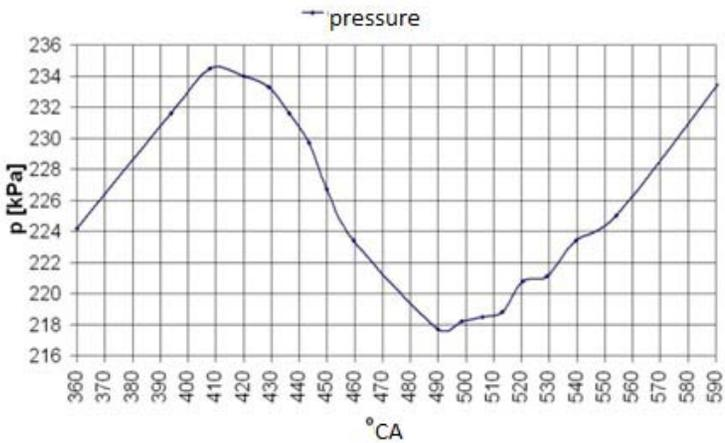
**Figure 3. 3.** Graph of pressure in the inlet system(filling)
