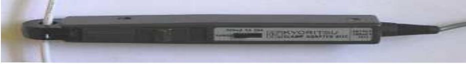
**Fig. 4. Current probe KYROYTSU model 8112, current ranges up to 200 mA/ 2 A/ 20 A, 40 Hz – 10 kHz, at the range of 200 mA the measuring constant is equal to 1 mA/mV**
