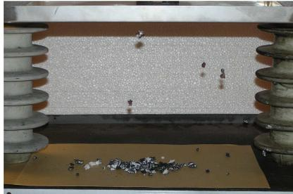
Fig. 5. The movement of conductive particles in DC field
