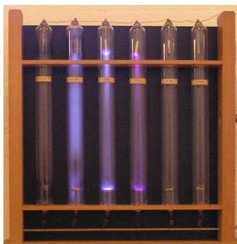
**Fig. 9. The gas ionization into three cylinders after application of AC voltage of 1100 V<sub>peak</sub> with the frequency of 5 kHz.**
