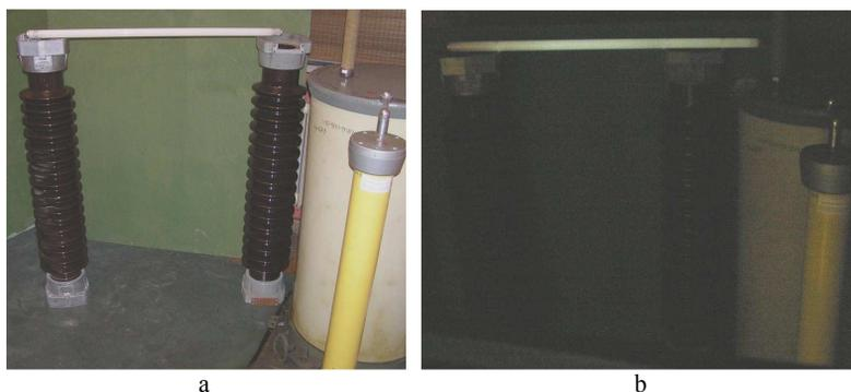
**Fig. 14. 120 cm long fluorescent tube in electric field of 110 kV transformer. a – mounting arrangement, b – light visible in semi-dark room**
