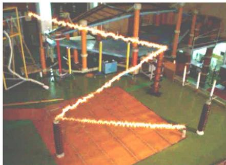
**Fig. 1. Exploding wire with the thickness of 0,04 mm and the length of 15 m in HV Laboratory of WUT**
