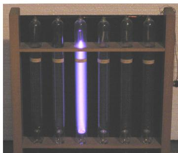
**Fig. 7. The light emission at the 50 Hz voltage of  $2700 V_{\text{peak}}$  in the cylinder with the  $p \cdot s$  product of 80 hPa-cm.**
