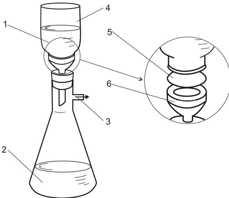
**Figure 4.4.** Membrane filtration system: 1 – filtered water, 2 – receiver flask, 3 – connection with water vacuum pump (outlet to vacuum pump), 4 – funnel, 5 – membrane filter, 6 – filter holder base.
