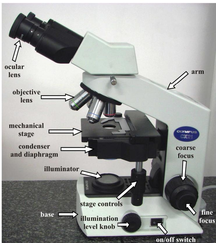
**Figure 1.2.** Components of a microscope.
