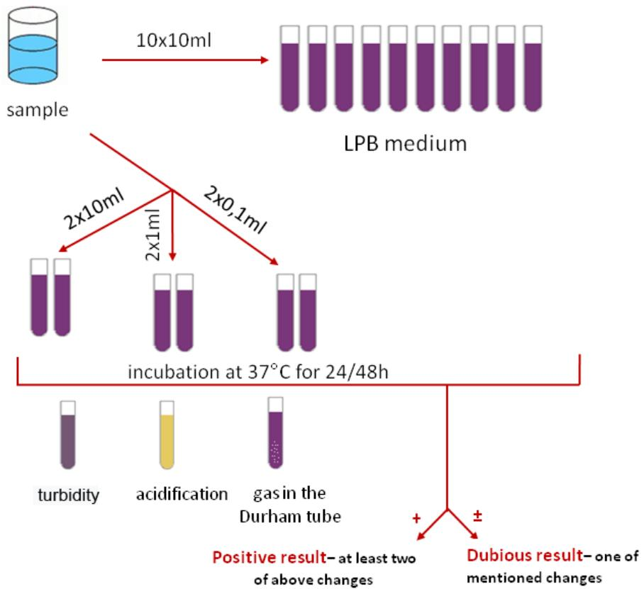
**Figure 4.1.** Multiple-tube Fermentation technique – presumptive test for coliforms.
