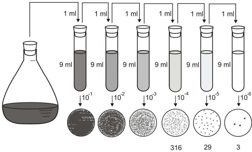
**Figure 3.6.** Plate count dilution procedure.
