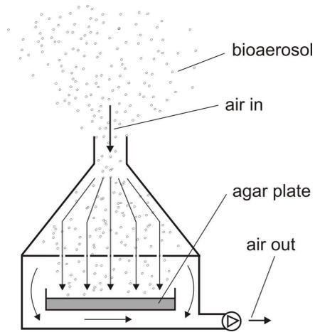
**Fig. 6.3.** Principle of the impact method.
