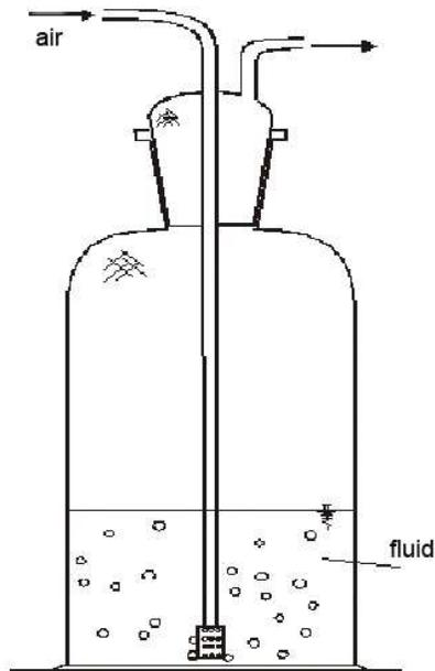
**Figure 6.2.** Washer bottle for bioaerosol absorption with the filtration method.
