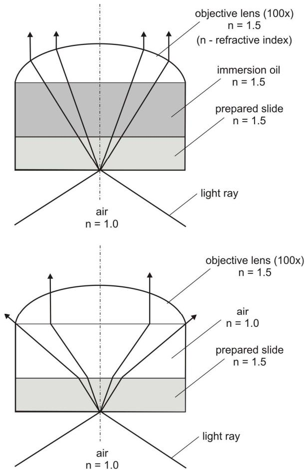
**Figure 1.3.** Principle of immersion microscopy.
