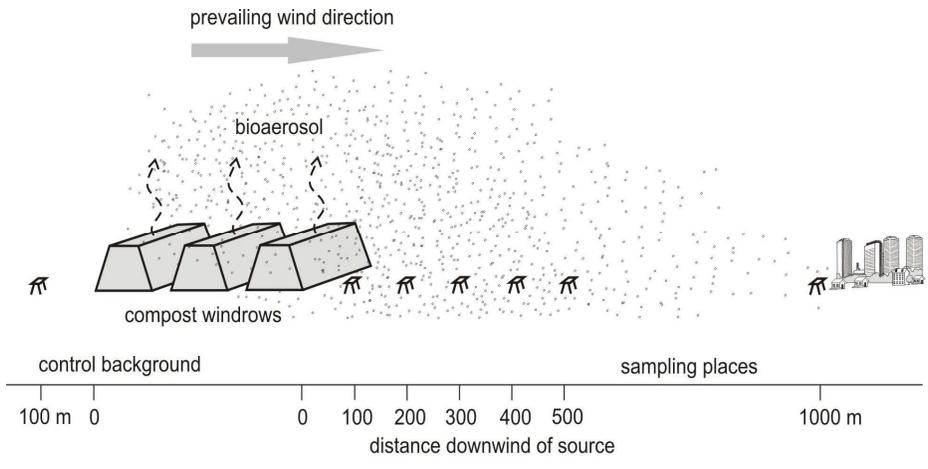
**Figure 6.5.** Investigation of the bioaerosol concentration near a composting plant.
