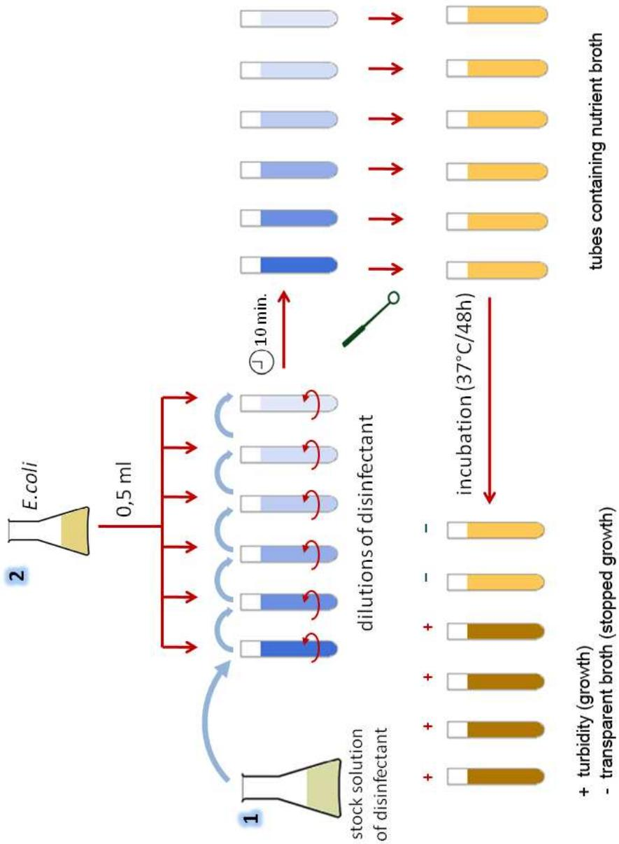
**Figure 2.1.** Scheme of determining the phenol coefficient.
