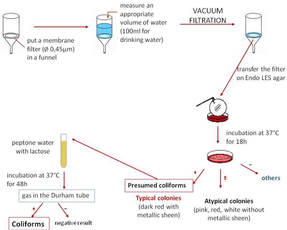
**Figure 4.6.** Membrane Filtration method for coliforms.
