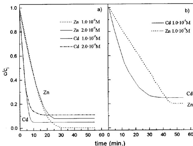
Fig. 1. Flotation curves for the Zn(II) and Cd(II) ions from solutions containing single metal (a) and equimolar metal mixture (b) by  $2.0 \cdot 10^{-4}$  M DBSNa
