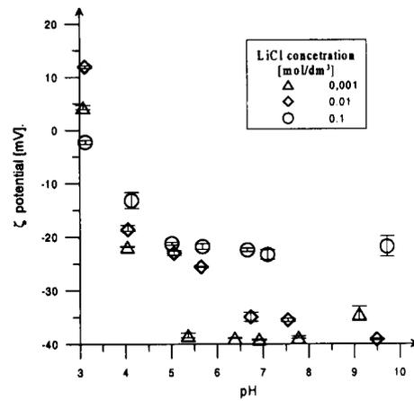
Fig. 4. Zeta potential as a function of pH and electrolyte concentration for the  $MnO_2/LiCl$  solution system
