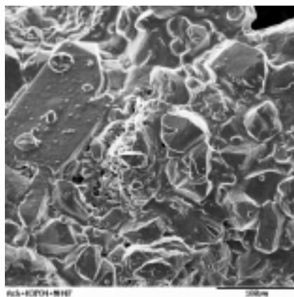
Fig 8. Asbestos after degradation process in solution (NH<sub>4</sub>F and H<sub>3</sub>PO<sub>4</sub>)
