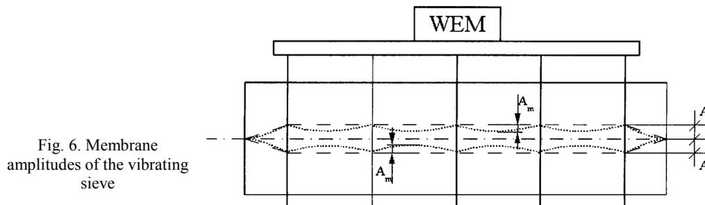
Fig. 6. Membrane amplitudes of the vibrating sieve
