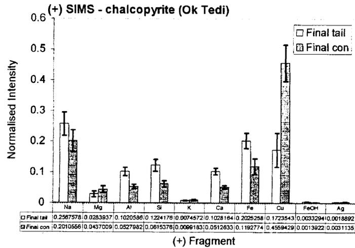
Fig. 7. (+) SIMS. Ok Tedi. Mass spectra for pyrite in the final tail and final concentrate (confidence intervals calculated for P=95%)
