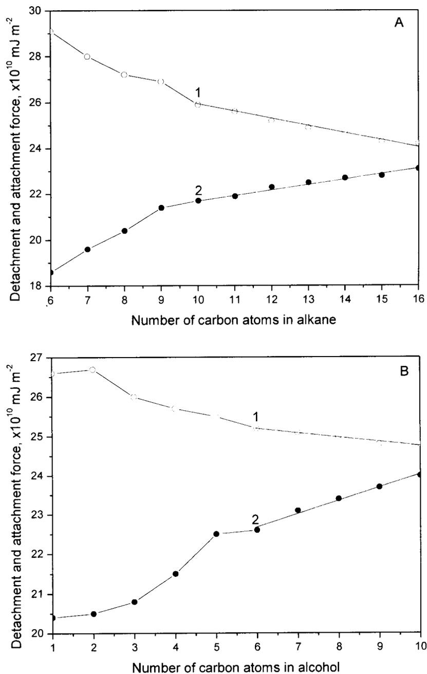
Fig. 2. The detachment (curve 1) and attachment (curve 2) forces as a function of the number of carbon atoms in molecule of alkanes (Fig. 2A) and alcohols (Fig. 2B)
