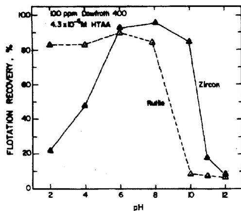
Fig. 6. Floatability of rutile and zircon with amine as a function of pH.
