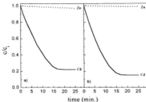
Fig. 2. Kinetic curves of the Zn(II) and Cd(II) ions from aqueous solutions containing 1.0 M bromide (a) and 1.0 M iodide (b) ions in solution by CPCl,  $[Zn^{2+}] = [Cd^{2+}] = 1.0 \cdot 10^{-5}$  M,  $[CPCl] = 2.0 \cdot 10^{-4}$  M, pH = 4.0
