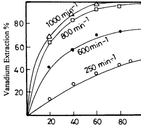
Fig. 6. Effect of speed agitation on vanadium extraction
