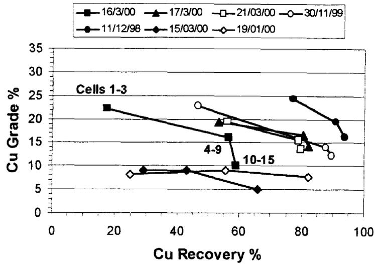
Fig. 1. Copper grade-recovery curves for rougher-scavenger surveys at Ok Tedi
