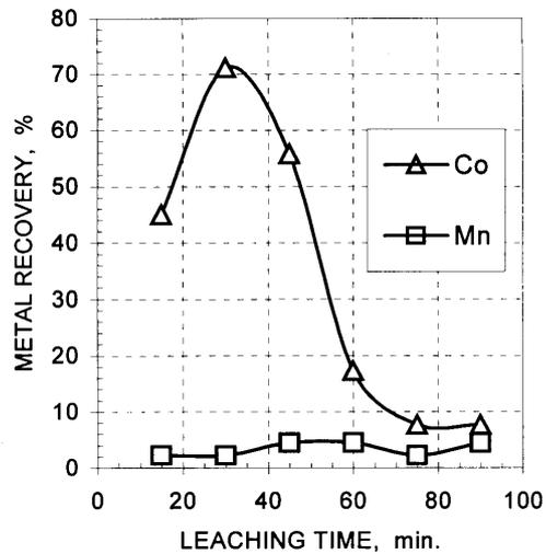
Figure 2. Recovery of Co and Mn during the leaching of nodules in NH<sub>3</sub> - SO<sub>2</sub> solution. (NH<sub>3</sub> · H<sub>2</sub>O - 0.6 M, (NH<sub>4</sub>)<sub>2</sub>CO<sub>3</sub> - 0.6M, flow rate of SO<sub>2</sub> -100 ml/min., temperature – 90 °C, stirring rate – 900 rpm, liquid/solid ratio - 10:1)
