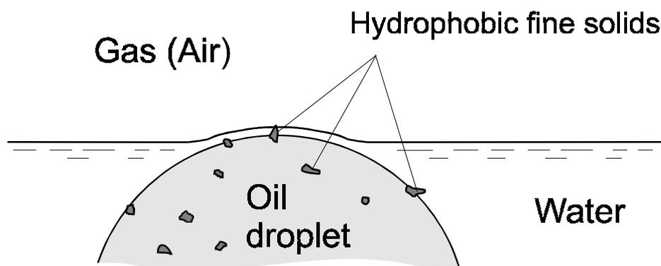
Figure 5. The pin-effect of fine protruding hydrophobic particles
