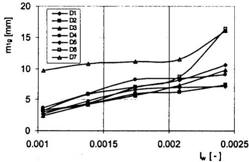
Fig. 4. The effect of wetting intensity during granulation on the value of  $m_{1g}$
