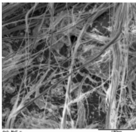
Fig 7. Asbestos after degradation process in solution (NaF)
