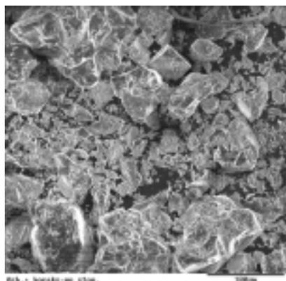
Fig 5. Asbestos fused with borax
