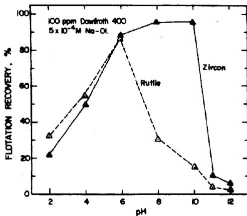
Fig. 5. Floatability of rutile and zircon with sodium oleate as a function of pH.
