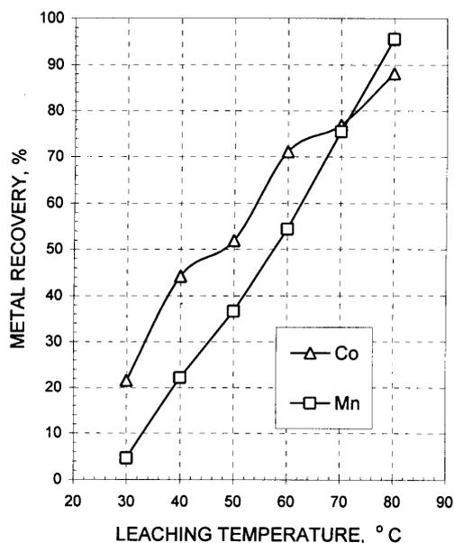
Fig. 8. Effect of leaching temperature on recovery of Co and Mn from nodules. (NaCl - 0.55 M, HCl - 3.0 M, leaching time - 1.5 hour, stirring rate - 900 rpm, liquid/solid ratio - 10:1)
