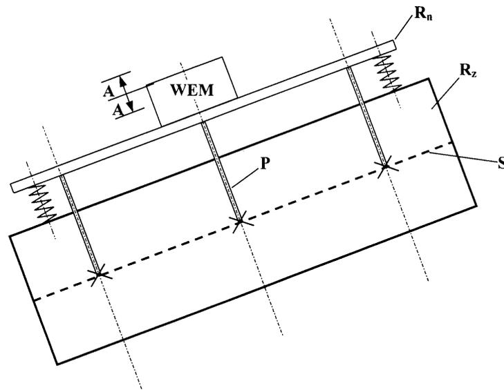
Fig. 4. Screen with a driving frame
