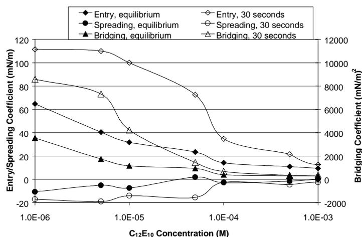
Figure 7. Entry, spreading and bridging coefficients of the system: C<sub>12</sub>E<sub>10</sub> aqueous solution and dispersed paraffin oil
