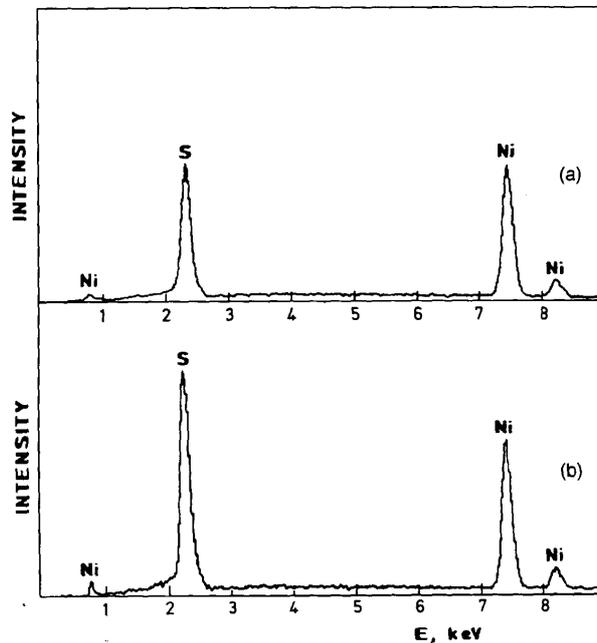
Fig. 3. Microprobe diagrams of the particle shown in Figure 2 for: grey phase (indicated by a circle), white phase (indicated by a cross)
