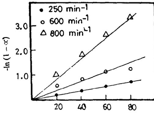
Fig. 8. Test of applicability of film diffusion model to the experimental data
