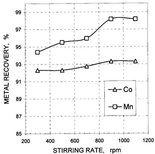
Fig. 6. Effect of stirring rate on recovery of Mn and Co from nodules (HCl + NaCl solution). (NaCl - 0.55 M, HCl - 5.0 M, temperature - 30 °C, liquid/solid ratio - 10:1, leaching time - 1.5 hour)
