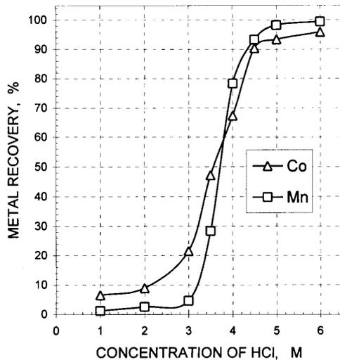
Fig. 5. Effect of concentration of hydrochloric acid on leaching recovery for Co and Mn.. (NaCl - 0.55 M, tem. - 30 °C, stirring rate 900 rpm, liquid/solid ratio - 10:1, leaching time - 1.5 hour)
