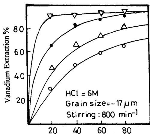
Fig. 3. Relation between vanadium extraction and time at different temperatures
