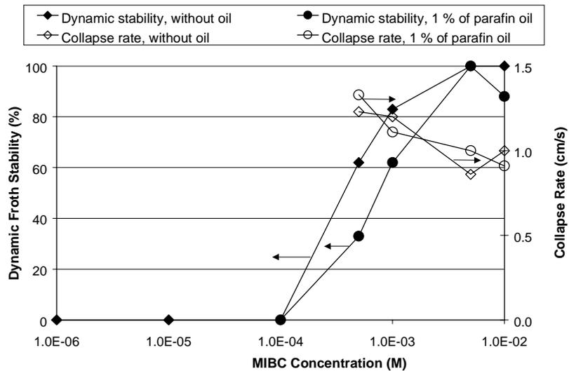
Figure 9. Dynamic stability and collapse rate of MIBC aqueous solutions
