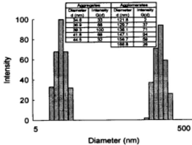
Fig. 2. Particle size distribution of TiO<sub>2</sub> modified with U-611 silane
