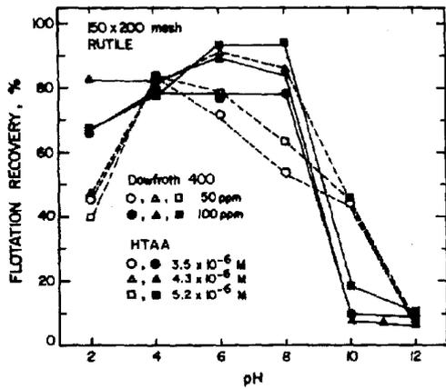
Fig. 3. Floatability of rutile with amine as a function of pH
