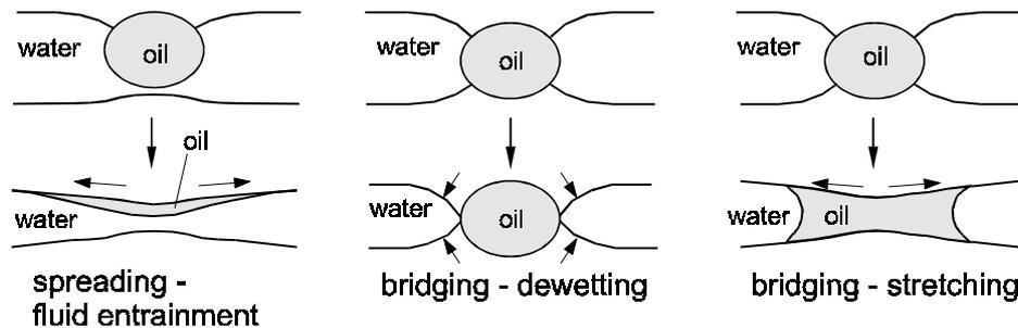
Figure 4. Three possible mechanisms of foam film destruction by an oil droplet, adopted from (Denkov et al. 1999)
