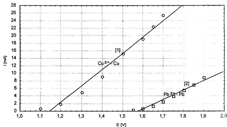
Fig. 1. Current – voltage dependence 1 – 40% solution  $\text{CH}_3\text{COONH}_4 + 5 \text{ g/dm}^3 \text{ Cu}(\text{CH}_3\text{COO})_2$
