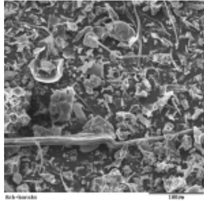
Fig 4. Asbestos fused with borax
