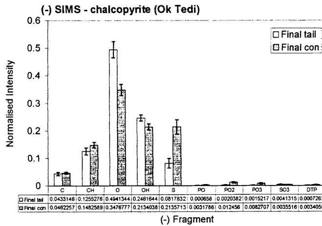
Fig. 8. (-) SIMS. Ok Tedi. Mass spectra for chalcopyrite in the final tail and final concentrate (confidence intervals calculated for P=95%)
