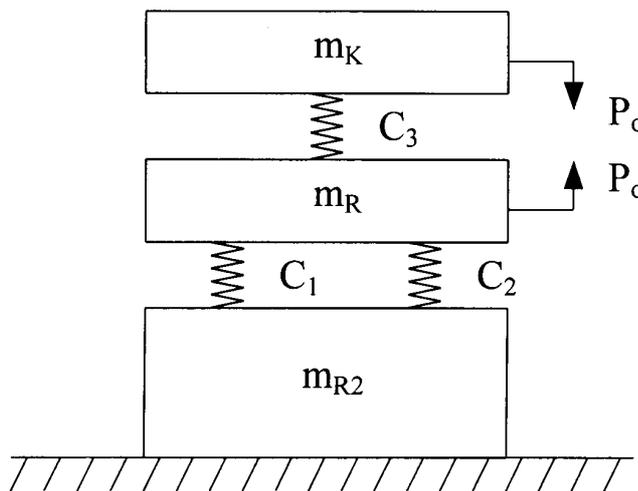
This system is characterised by variable flexibility constant  $C_2$ . During the screen operation the sieve is “elongated” (deformed), which leads inevitably to changes in the sieve elasticity. So, to make typical dynamic calculations of the vibrating system is difficult because:
