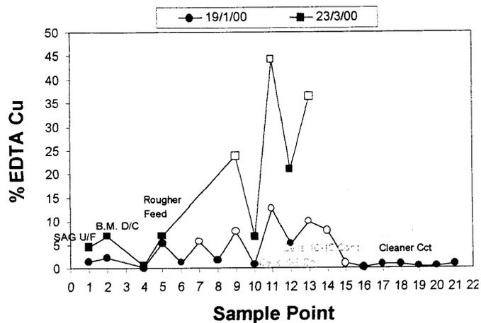
Fig. 4. Examples of EDTA extraction surveys, showing % EDTA Cu for plant streams. Tailings streams are shown in white
