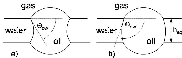
Figure 3. Oil bridging. a) unstable bridge,  $\Theta_{ow} \leq \pi/2$ , b) stable bridge,  $\Theta_{ow} > \pi/2$ , adopted from (Denkov 1999)
