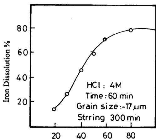
Fig. 9. Effect of temperature on iron dissolution
