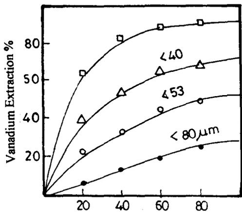
Fig. 7. Effect of particle size on vanadium extraction
