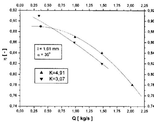
Fig. 11. Screening efficiency as a function of capacity for sharp-edged particles
