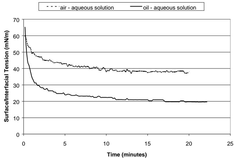
Figure 8. Surface/interface tension of  $1 \times 10^{-5}$  M  $C_{12}E_{10}$  as a function of time
