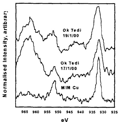
Fig. 5. XPS  $\text{Cu}_{2p}$  spectra for Ok Tedi rougher feed compared to MIM Cu
