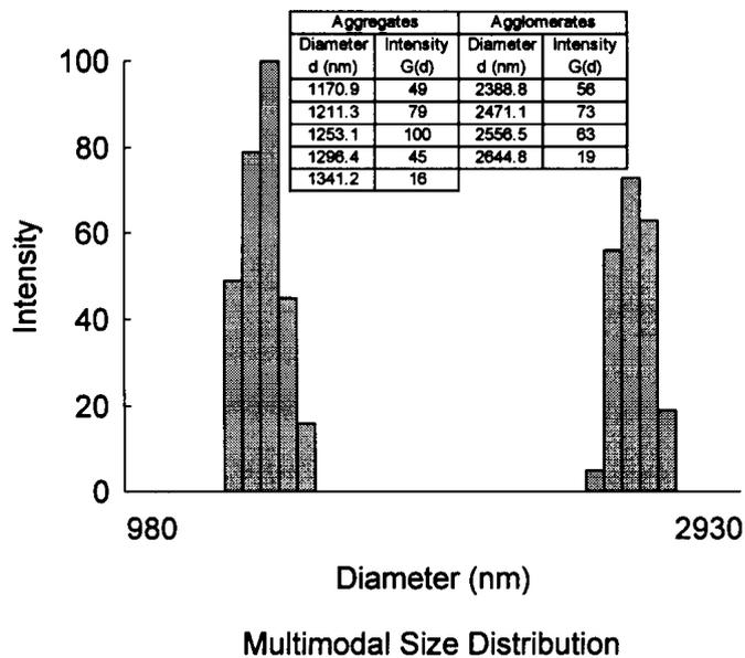
Fig. 1. Particle size distribution of unmodified carbonate-silicate filler
