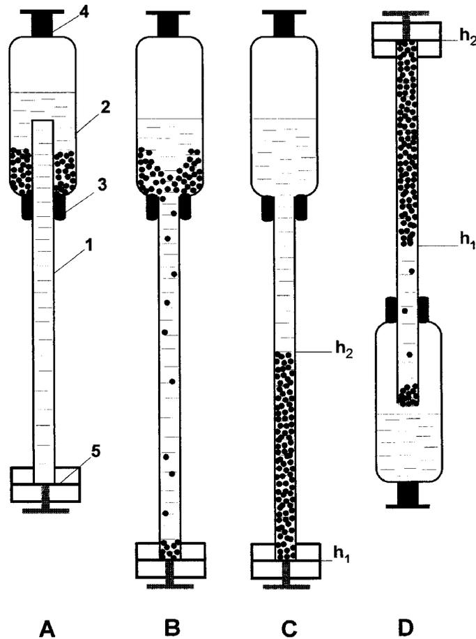
Fig. 1. Schematic diagram of the device for the destruction time measurements: (1) glass tube; (2) glass vessel; (3) rubber plug; (4) stopper; and (5) sealing system. (A) The device filled with the studied suspension; (B) formation of the sediment column; (C) the sediment column formed; (D) destruction sediment column structure.  $h_1$  and  $h_2$  are the bottom and upper levels of the of the sediment column
