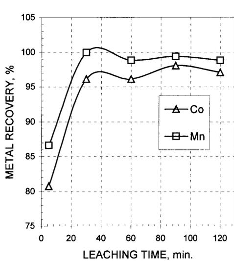
Fig. 3. Recovery of Co and Mn during the leaching of nodules with hydrochloric acid solution. (HCl – 6.0 M, temperature – 30 °C, stirring rate - 900 rpm, liquid/solid ratio - 10:1)
