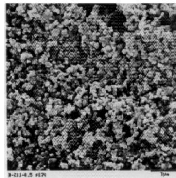
Fig. 3. a) Particle size distribution and b) SEM of TiO<sub>2</sub> modified with A-174 silane
