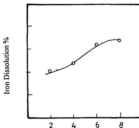
Fig. 10. Effect of hydrochloric acid concentration on iron dissolution
