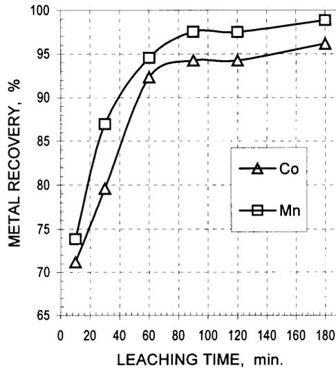
Fig. 4. Recovery of Co and Mn from nodules during the leaching in HCl + NaCl solution. (NaCl 0.55 M, HCl 5M, stirring rate 900 r/min., temperature 30°C, liquid to solid ratio 10:1)
