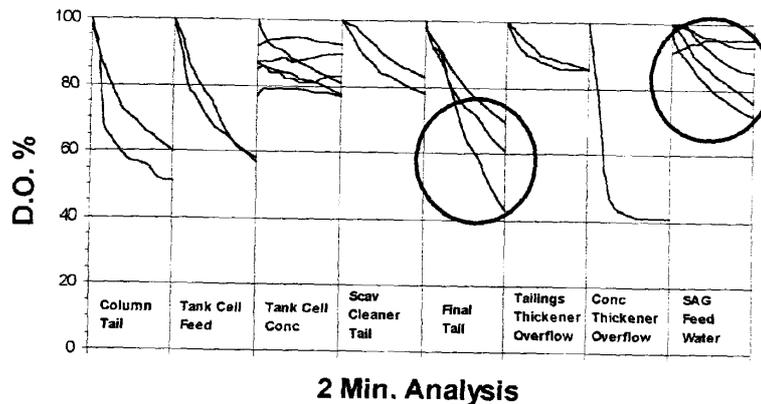
Fig. 3. Dissolved oxygen (D.O.) readings as % saturation taken over two minutes immediately after pulp sampling, during Ok Tedi surveys
