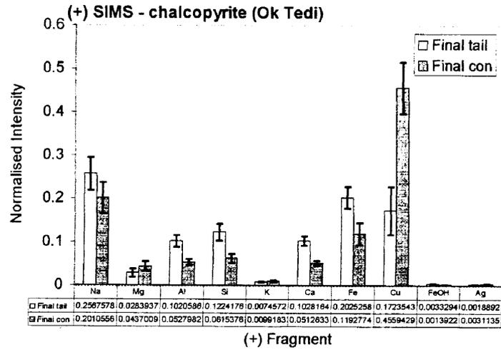
Fig. 6. (+) SIMS. Ok Tedi. Mass spectra for chalcopyrite in the final tail and final concentrate (confidence intervals calculated for P=95%)
