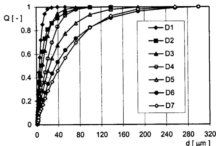
Fig. 1. Comparison of particle size distributions of fine-grained raw materials
