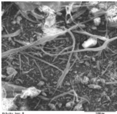
Fig 3. Asbestos fused with  $\text{H}_3\text{BO}_3$
