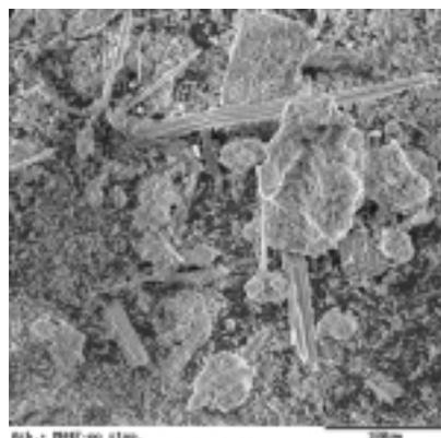
Fig 6. Asbestos fused with NH<sub>4</sub>F
