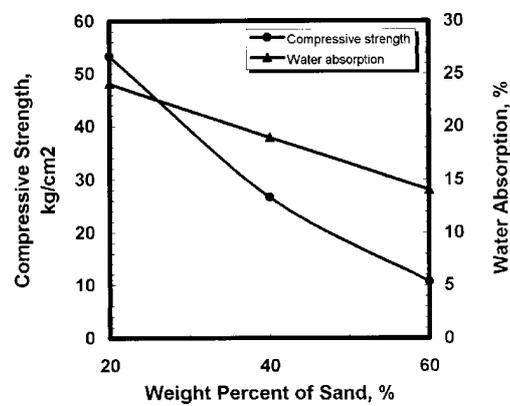
Figure 2. Effect of weight percent of sand (-1500 + 0  $\mu\text{m}$ ) on physical and mechanical properties of produced bricks
