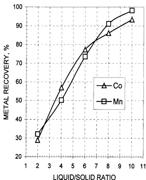
Fig. 7. Effect of liquid/solid ratio on recovery of Co and Mn. (NaCl - 0.55 M, HCl - 5.0 M, temperature - 30 °C, stirring rate - 900 rpm, leaching time - 1.5 hour)
