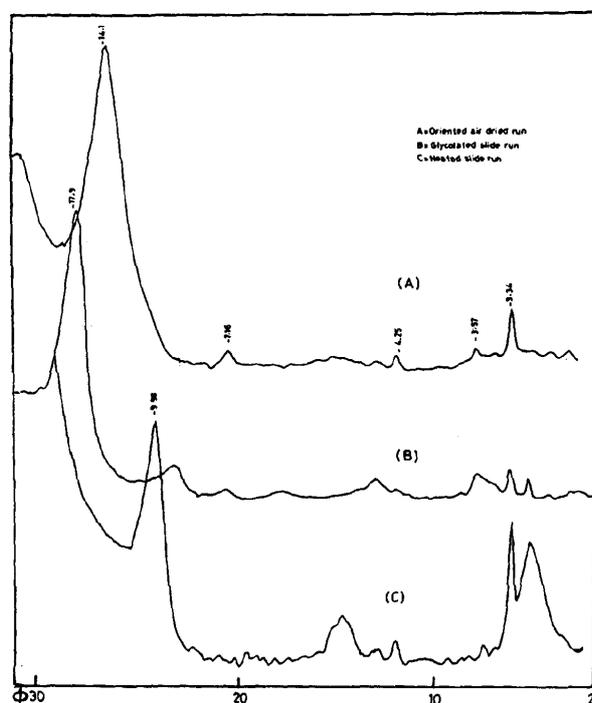
Fig. 2. Representative diffractogram of the clay fraction Abu Tartur black shale
