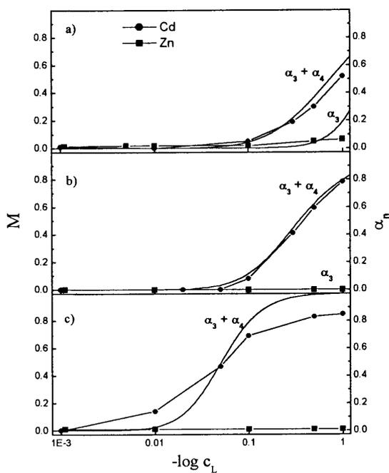
Fig. 3. Influence of analytical concentration of chloride (a), bromide (b) and iodide (c) on removal of Zn(II) and Cd(II) ions with CPCl, and molar fractions of anionic metal complexes, pH = 4.0
