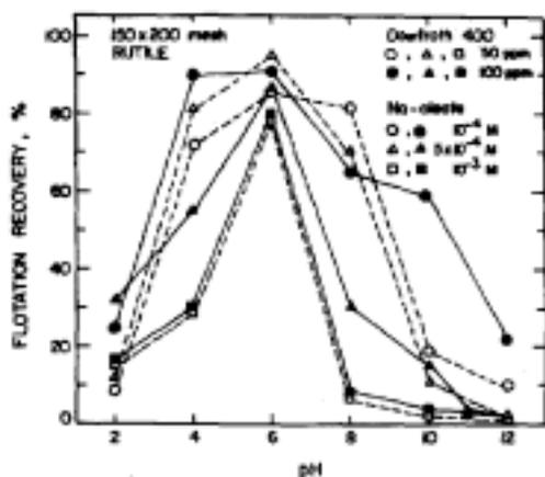
Fig. 1. Floatability of rutile with sodium oleate as a function of pH
