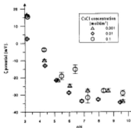
Fig. 6. Zeta potential as a function of  $\text{pH}$  and electrolyte concentration for the  $\text{MnO}_2/\text{CsCl}$  solution system.
