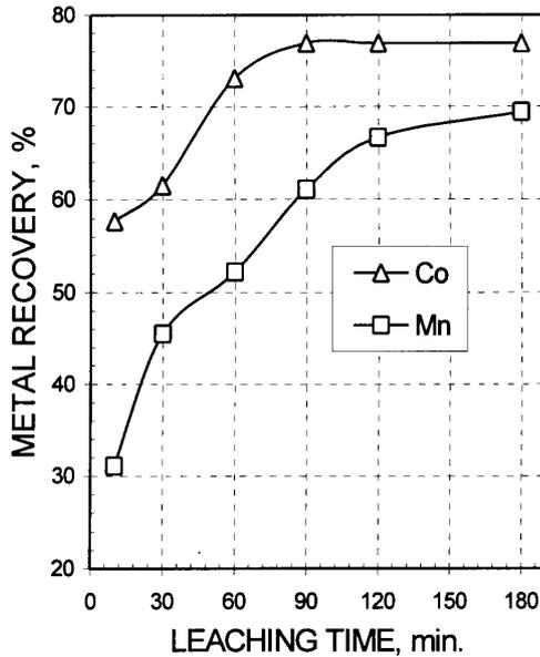
Fig. 1. The recovery – time relationship for HCl - NaCl leaching of nodules (NaCl - 4.0 M, HCl - 2.75 M, temperature – 30 °C, stirring rate - 900 rpm, liquid/solid ratio - 10:1)
