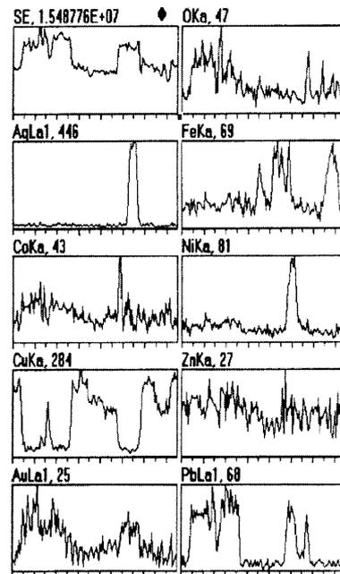
Fig.7. Distribution of O, Ag, Fe, Co, Ni, Cu, Zn, Au, Pb in the copper matte alongside profile A-B marked in fig. 6
