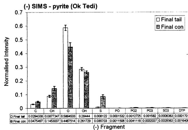
Fig. 9. (-) SIMS. Ok Tedi. Mass spectra for pyrite in the final tail and final concentrate (confidence intervals calculated for P=95%)
