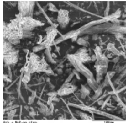
Fig 2. Asbestos fused with NaF (500 °C, 2h)
