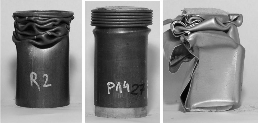
Fig. 14. Elements after deformation: a) round with single wall, empty, b) round with single wall filled with the foam whose density is 119.7, c) rectangular with single wall filled with the foam whose density is 119.7
