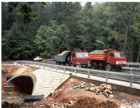
Fig. 4. View of bridge during tests under load scheme III in test stage II
