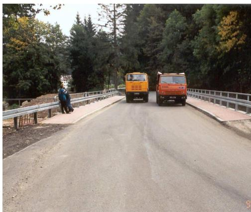
Fig. 5. View of bridge during tests under load scheme III in test stage III
