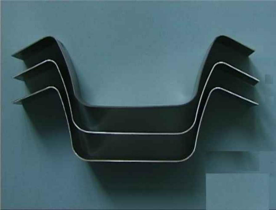
Fig. 3. The shape of aluminium alloy parts after spring-back
