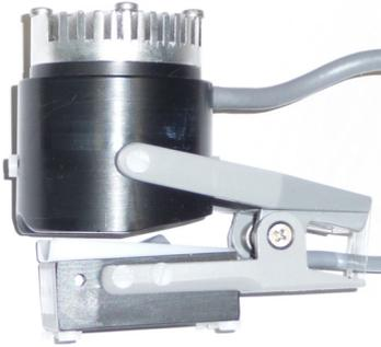
Fig. 7. LED and light sensor probes in the holding fixture.
