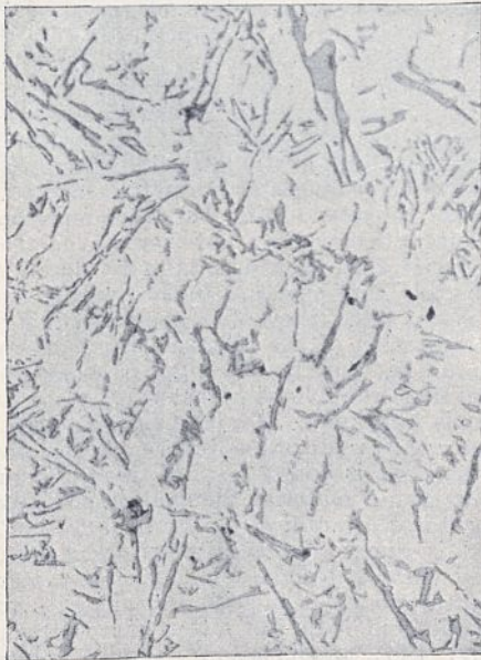
Fig. 3.—10.0 per cent. silicon. Centre of ingot. \times 150 .
