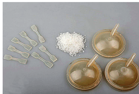
Fig. 12. Polymeric granules, injection molded samples for mechanical testing (type 5A, ISO 527) and pneumatic elements of the pump obtained from 50-50 PET-DLA copolymer
