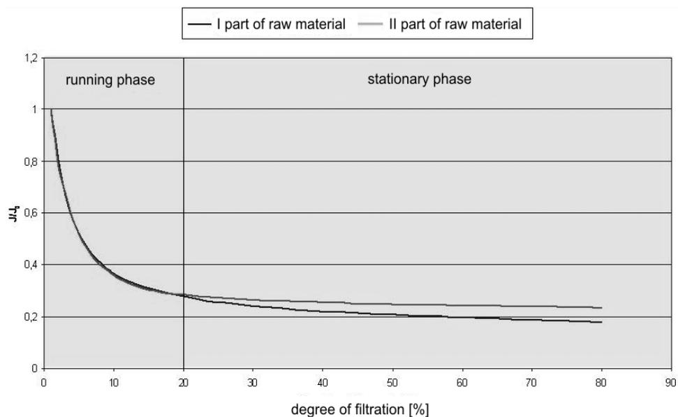
Fig. 1. Typical normalized filtrate flux for two batches of raw material
