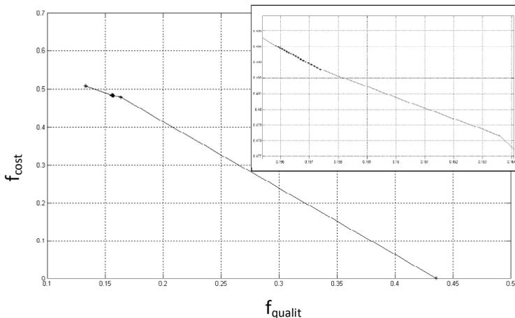
Fig. 3. Quality of a product in function of a production cost. Increment of a quality reply to the decreasing values in abscissal axis
