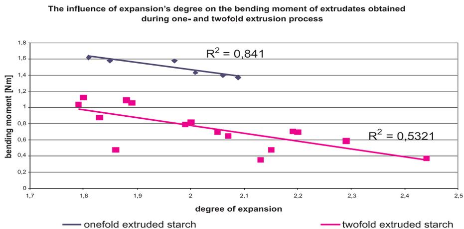
Fig. 1. The influence of expansion's degree on the bending moment of extrudates obtained during one- and twofold extrusion process
