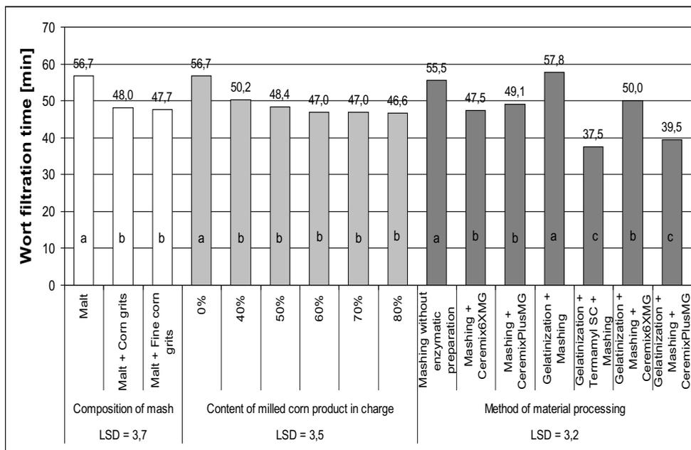
Fig. 2. Time of worts filtration in relation to the type and content of material in charge and to a processing method
