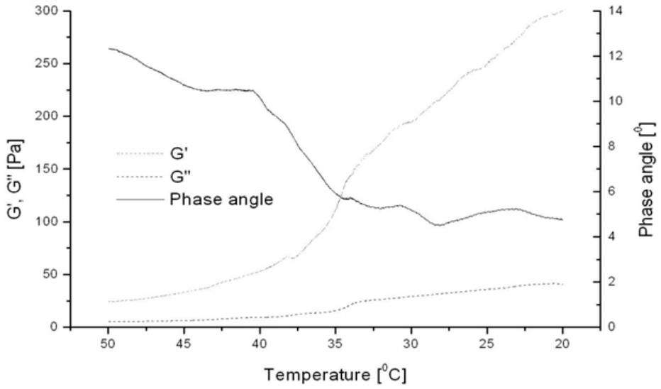
Fig. 15. Cooling curves of protein 4% and carrageenan 1%
