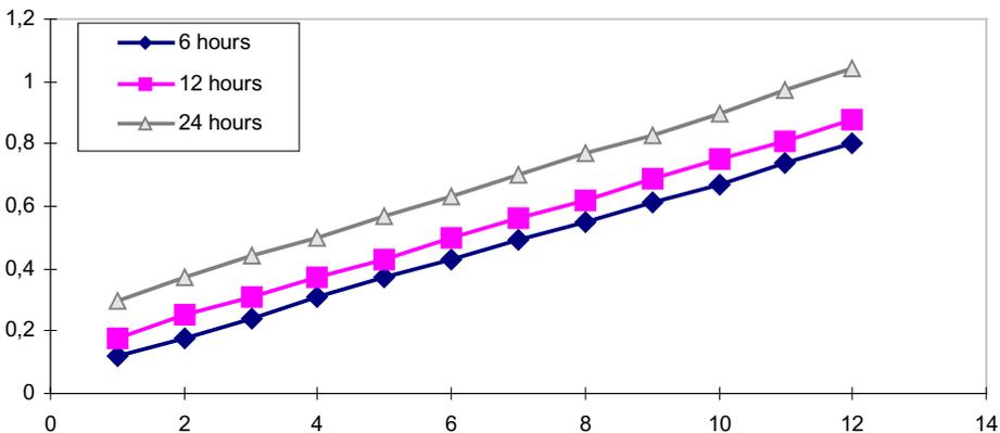
Fig. 1. Potato mass losses  $\Delta m$ , cooling them to  $6^\circ\text{C}$  at the temperature difference  $\Delta\Theta$
