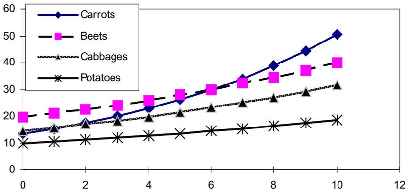
Fig. 3. Dependence of vegetable breathing heat  $q$  ( $W/t$ ) on their temperature  $T$  ( $^{\circ}\text{C}$ )
