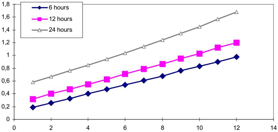
Fig. 2. Carrot mass losses  $\Delta m$ , cooling them to  $6^{\circ}\text{C}$  at the temperature difference  $\Delta\Theta$
