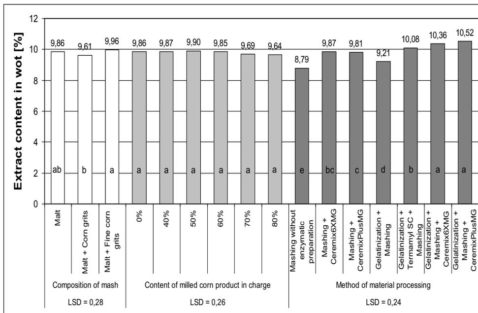
Fig. 3. Content of extract in worts in relation to the type and content of material in charge and to a processing method
