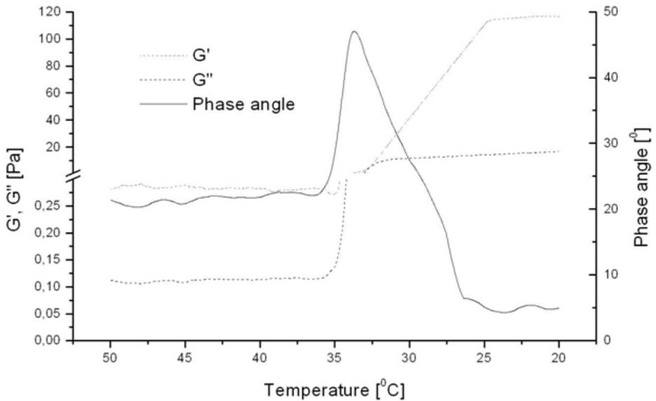
Fig. 14. Cooling curves of protein 4% and carrageenan 0,5%
