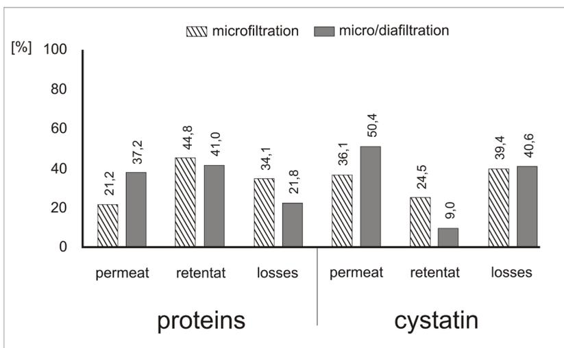
Fig. 2. Recovery of protein and active cystatin after microfiltration (MF) and micro/diafiltration (MFD) processes
