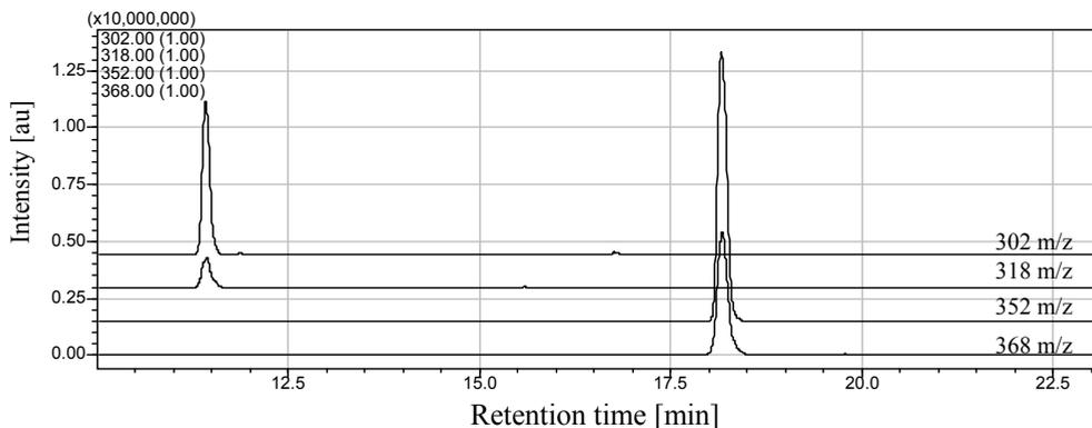
Fig. 2. ESI/MS chromatogram of desulfosinigrin (RT=11,40 min) and desulfoglucotropaeoiln (RT=18,15) in positive (b) mode
