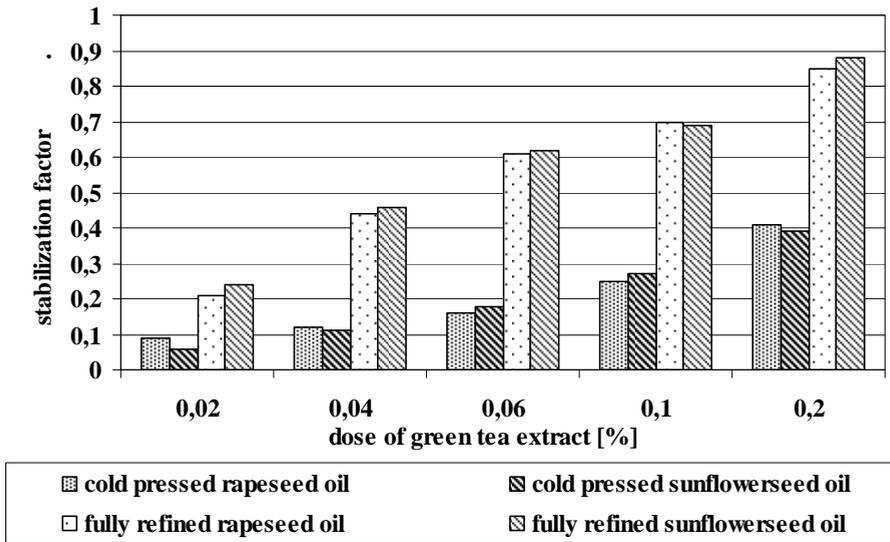
Fig. 1. Effects of green tea extract on stabilization factor of rapeseed and sunflower cold pressed oils and fully refined oils
