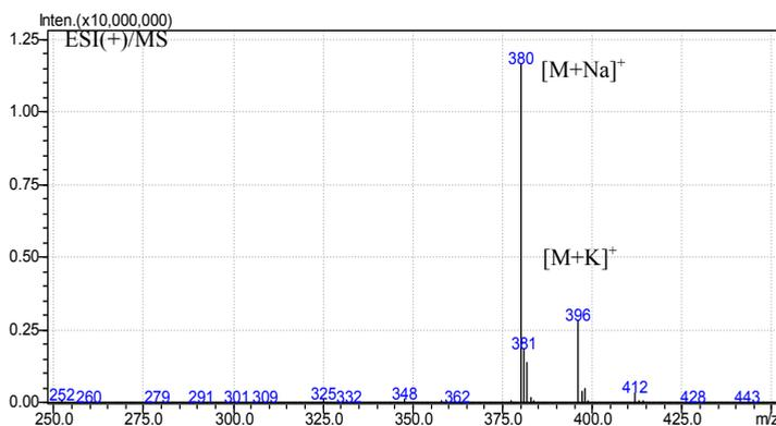
Fig. 3. ESI/MS spectra of desulfoglucoraphanin in negative and positive mode
