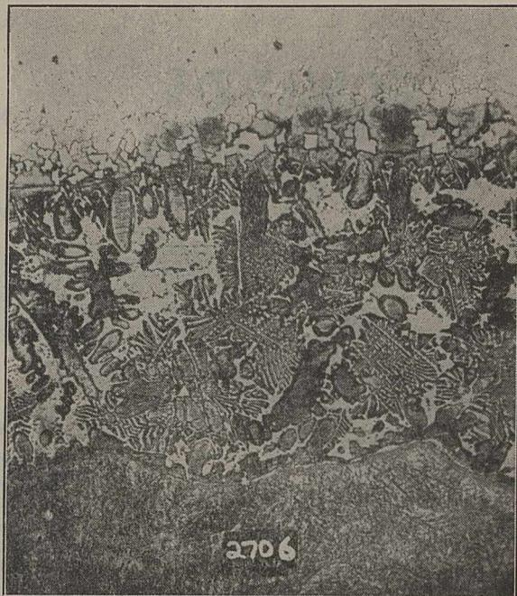
Section across junction of high-speed steel tip and plain carbon steel tool shank using Stalweld Powder as bonding material. (x 500)
