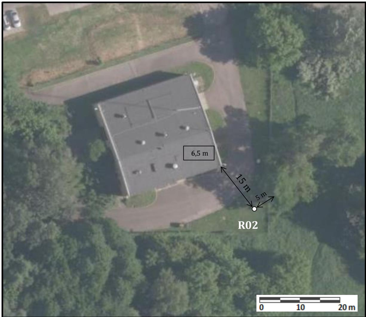
**Figure I.2.** Location site of rain gauge R02 of the Warsaw rain gauge network (in Rudzka St.)
