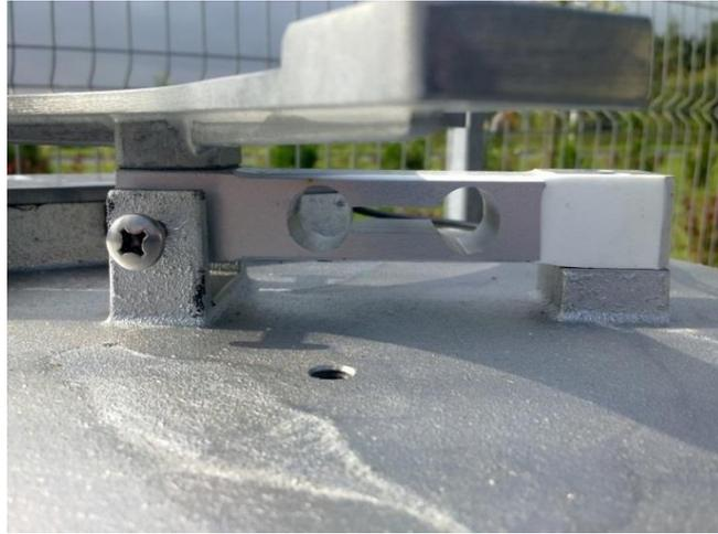
**Figure 3.8.** The strain-gauge bridge of an electronic weighing-type rain gauge
