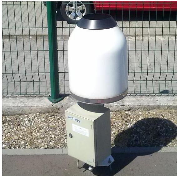
**Figure 3.7.** A MPS System weighing-type rain gauge
