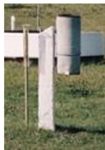
**Figure 3.2.** Hellmann rain gauges
