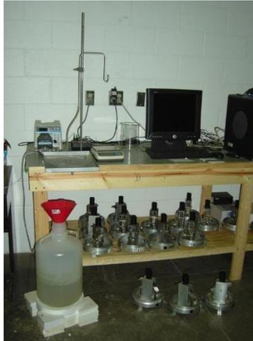
**Figure 3.4.** Measuring set used to rain gauge calibration at IIHR – Hydrosience & Engineering laboratory, Iowa State University (USA) (Licznar et al., 2013)
