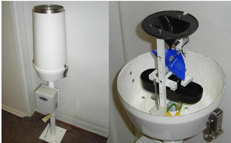
**Figure 3.3.** Tipping-bucket rain gauge. From the outside (on left) and from the inside (on the right)
