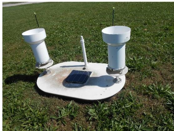
**Figure 3.9.** Tipping-bucket rain gauges
