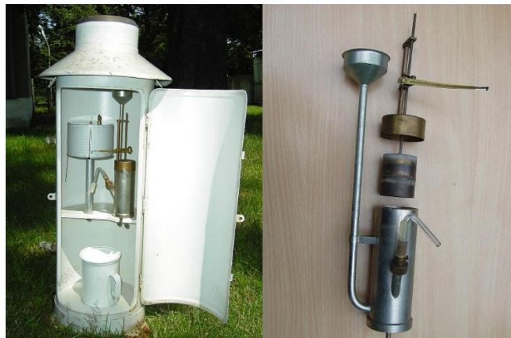
**Figure 3.5.** Siphon rain gauge in field (on left) and (on right) the inside elements. From the top: the funnel, the recording pen, the floating element and the siphon
