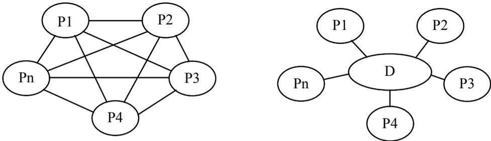
**Figure 1.** Graphic display of a peer-to-peer network (left) and a single-entity dominated network (right)
