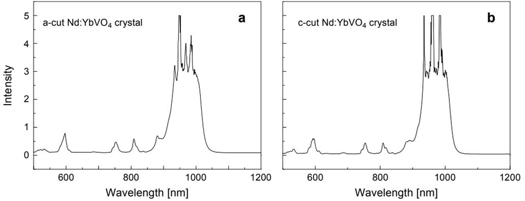
Fig. 1. Absorption spectrum of *a*-cut (a) and *c*-cut (b) Nd:YbVO<sub>4</sub> crystal.
