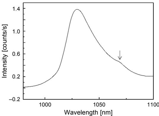
Fig. 5. The luminescence spectrum of Nd:YbVO<sub>4</sub> crystal stimulated by  $940 \text{ nm}$  light.
