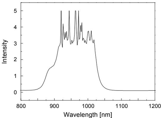
Fig. 2. Absorption spectrum of a pure YbVO<sub>4</sub> crystal.
