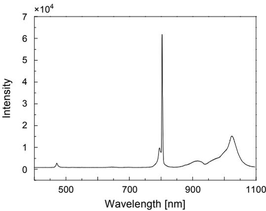
Fig. 3. The fluorescence spectrum of Nd:YbVO<sub>4</sub> crystal stimulated by 808 nm light.
