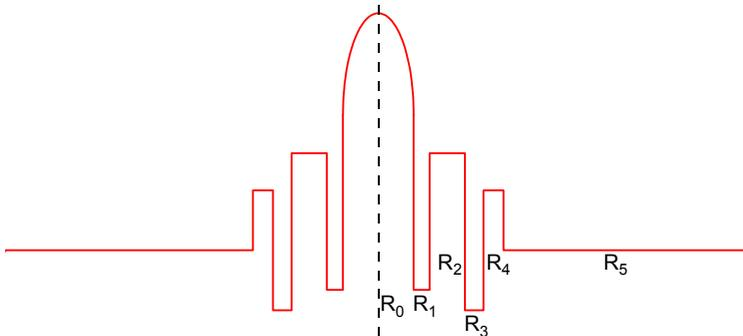
Fig. 1. Refractive index profile of our optimized NZDSF.
