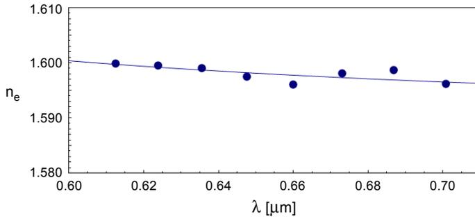
Fig. 11. Profile of extraordinary refractive index for 1292.
