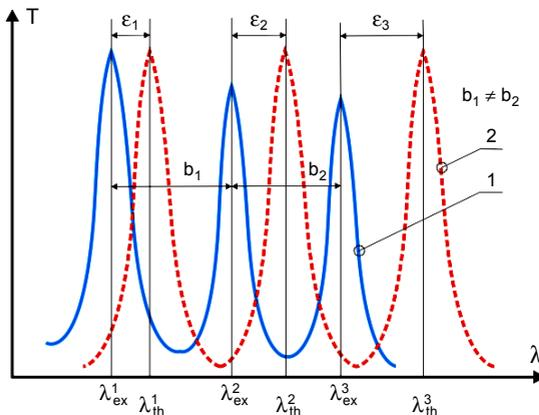
Fig. 4. Positions of interference maxima from experimental transmittance for three peaks (curve 1) and position of theoretical peaks of transmittance (curve 2);  $\epsilon$  denotes distance between the maxima of theoretical and experimental transmittance.
