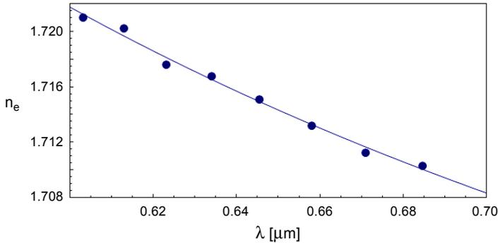
Fig. 7. Profile of extraordinary refractive index for 5CB.
