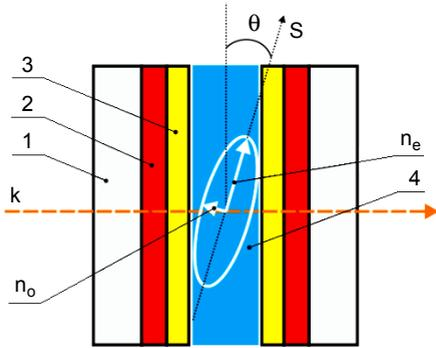
Fig. 2. Structure of plates of FPF filled by NLC with homogenous texture; 1 – glass plates, 2 – ITO electrodes, 3 – polyimide layers, 4 – liquid crystal layer,  $\mathbf{k}$  – wave vector direction,  $S$  – director,  $\theta$  – deviation angle of the director.
