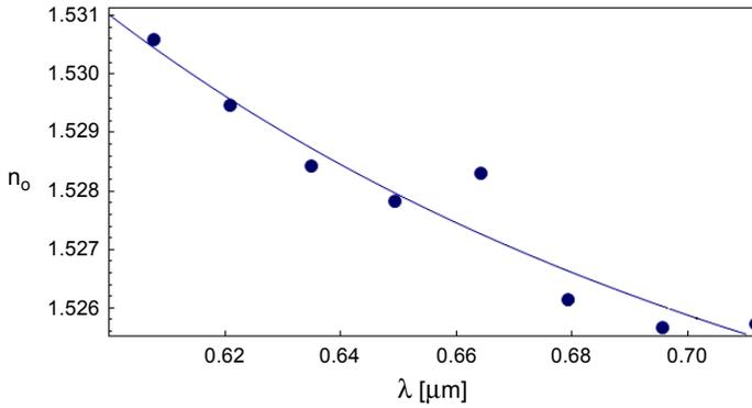
Fig. 5. Profile of ordinary refractive index for 5CB.
