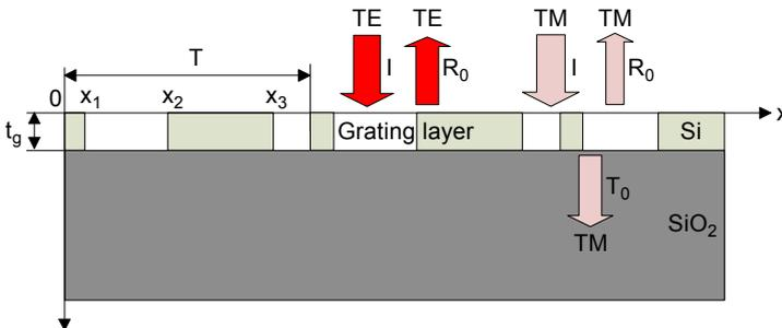
Fig. 1. Schematic of a grating PSBS. We denote  $T$ ,  $t_g$ ,  $x_1$ ,  $x_2$  and  $x_3$  as the grating period, thickness, and transition points, respectively. The incidence medium is air, and the substrate is silica. The refractive indices are:  $n_{\text{air}} = 1.0$ ,  $n_{\text{Si}} = 3.48$ ,  $n_{\text{silica}} = 1.47$ .
