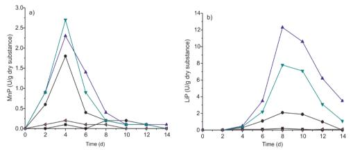
Fig. 5. Time dependences of MnP (a) and LiP (b) activities of SSF with the sludge pretreated under various doses of H<sub>2</sub>O<sub>2</sub> (in cm<sup>3</sup>/2 kg of sludge):  $\blacksquare -10$ ,  $\bigstar -200$ ,  $\bigstar -200$ ,  $\blacktriangledown -300$ , and  $\blacktriangleleft -400$
