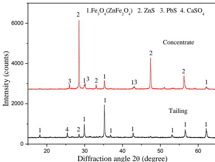
Fig. 9. XRD patterns of flotation concentrate and tailing
