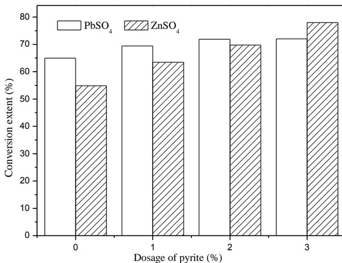
Fig. 6. Effect of pyrite dosage on conversion extent
