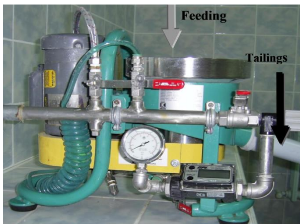
Fig. 4. Lab-scale batch Knelson concentrator
