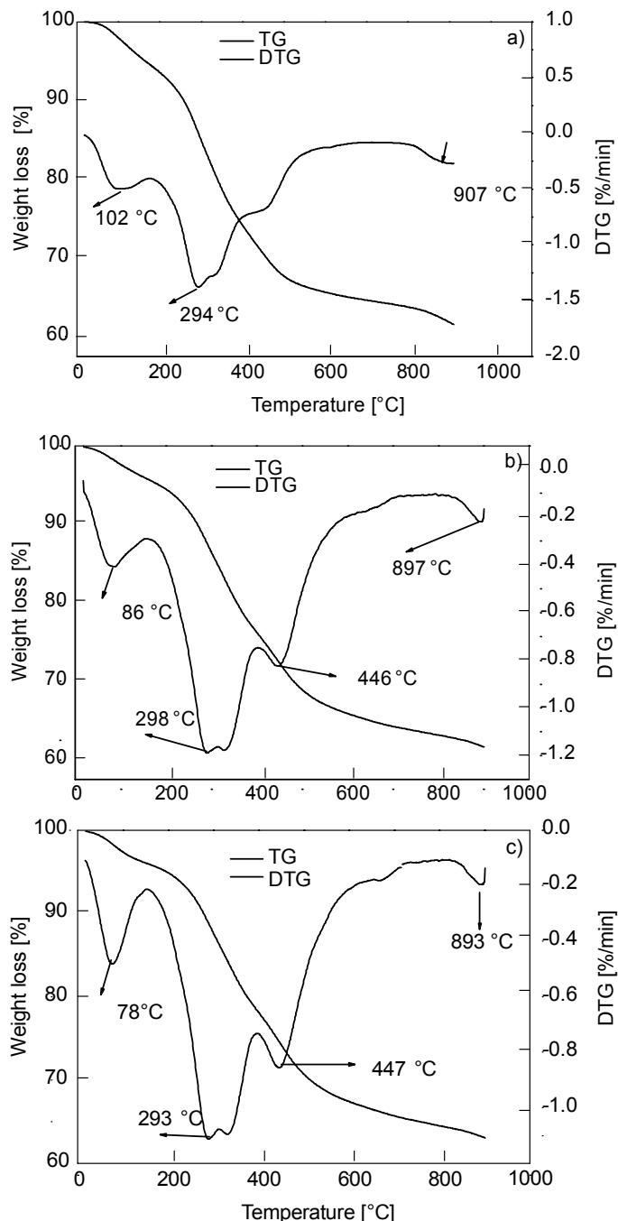
Fig. 2. Results of TG and DTG for the samples: a) sludge, b) sludge and coal, c) sludge briquettes (heating rate – 10 °C/min, N<sub>2</sub> flow rate – 35 cm<sup>3</sup>/min)
