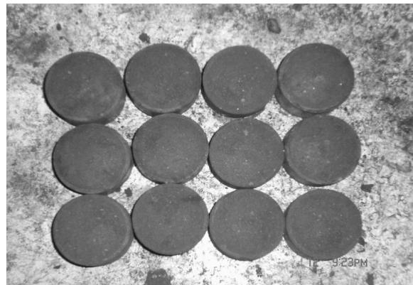
Fig. 1. Shape and size of sludge briquettes; diameter 30 mm, height 20 mm
