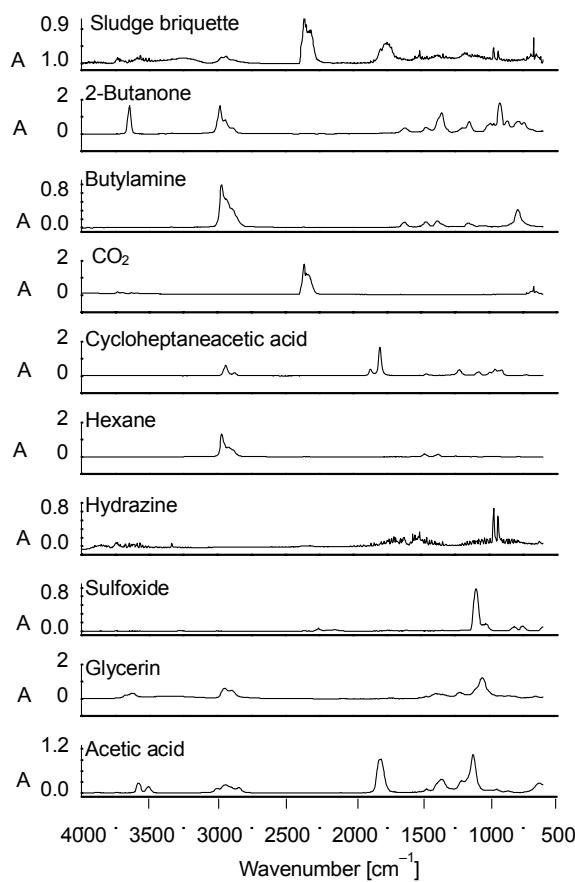
Fig. 3. Identification of pyrolysis of sludge briquettes at the second DTG peak (290 °C); A – absorbance
