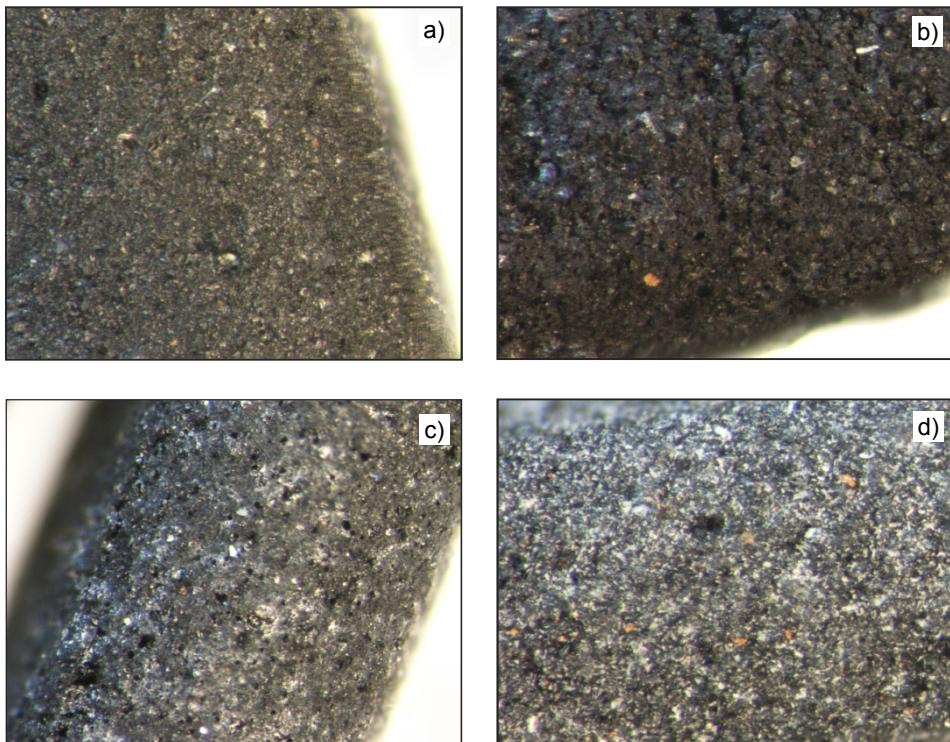
Fig. 4. Images of the external surfaces of: virgin granulated activated carbon, WDex (a), regenerated carbons, WDex/Fe<sup>2+</sup>/H<sub>2</sub>O<sub>2</sub> (b) and WDex/Fe<sup>2+</sup>/Ox (c), magnification 80×
