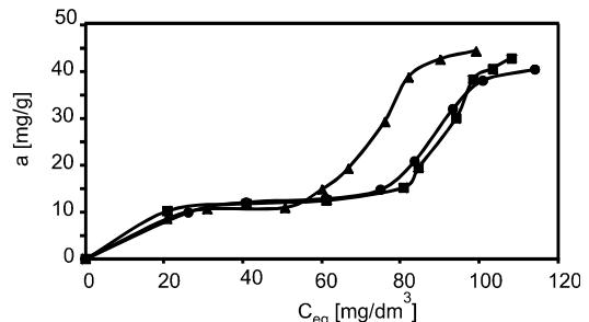
Fig. 2. Sorption isotherms of crystal violet on virgin and regenerated activated carbons:
