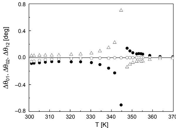
Fig. 1. Temperature dependences of differences among the characteristic azimuthal angles  $\Delta\theta_{01}$  (●),  $\Delta\theta_{02}$  (○),  $\Delta\theta_{12}$  (△) for the CGG crystals as measured for one of the orientations of specimen in the PSA system at 780 nm.
