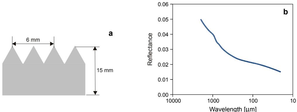
Fig. 5. Properties of emitter plate of the differential THz blackbody: dimensions (a), spectral reflectance (b).
