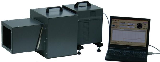
Fig. 7. Photo of the test system for testing passive surveillance THz imagers.
