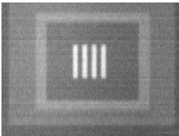
Fig. 8. Image of the THP test system generated by the tested THz imager during MRTD measurements (tests of a scanning 64-element imager).
