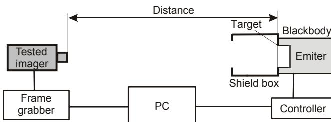
Fig. 3. Diagram of the variable distance test system.
