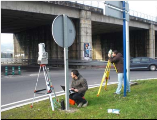
Fig. 1. RIEGL LMS Z390i during surveying process.
