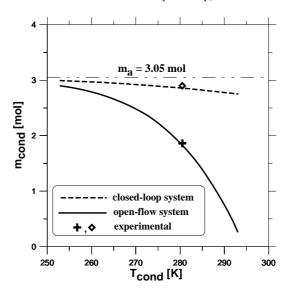
Fig. 3. Comparison of simulation and experimental results for the recovery of isopropanol in TSA systems with closed-loop and open-flow regeneration
