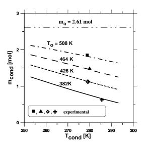
Fig. 2. Simulation and experimental results for the recovery of toluene in TSA system with closed-loop regeneration ( $m_a$  is the amount of organic compound adsorbed at the end of adsorption step)
