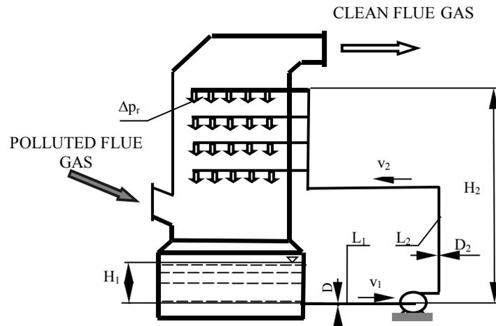
Fig. 1. Circulation of absorption slurry in the system: slurry reservoir – the highest level of slurry spraying in absorber
