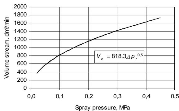
Fig. 2. Characteristic curve of work of eccentric atomizer of  $\text{CaCO}_3$  slurry
