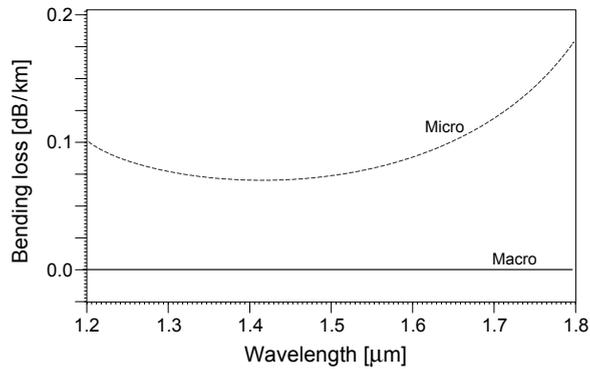
Fig. 11. Variations of bending loss via wavelength of our optimized fiber.
