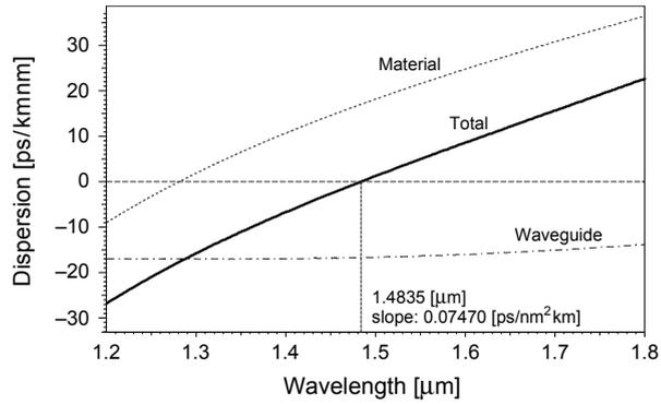
Fig. 3. Variations of dispersion vs. wavelength due to the addition of region  $R_2$  in refractive index profile.
