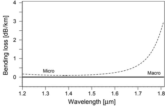
Fig. 5. Variations of bending loss vs. wavelength due to the addition of region  $R_2$  in refractive index profile.
