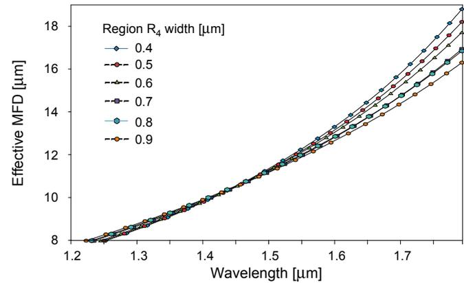
Fig. 20. Effective MFD vs. wavelength.
