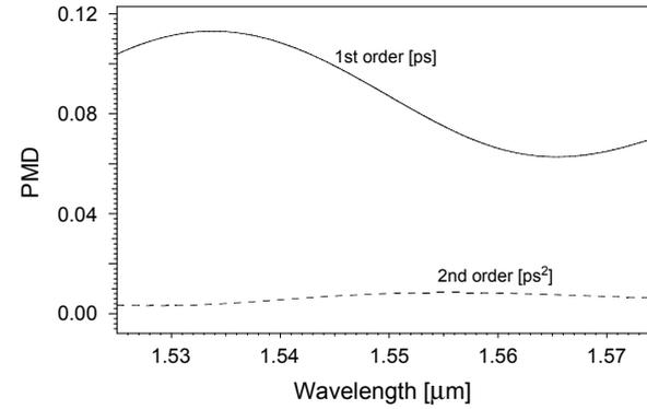
Fig. 4. Variations of PMD vs. wavelength due to the addition of region  $R_2$  refractive index profile.
