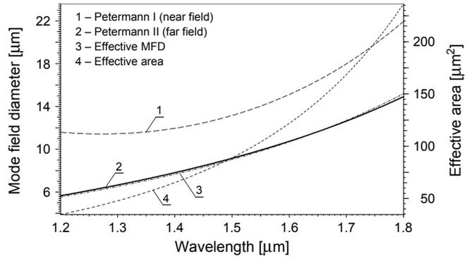
Fig. 9. Variations of effective area and MFD vs. wavelength of our optimized fiber.
