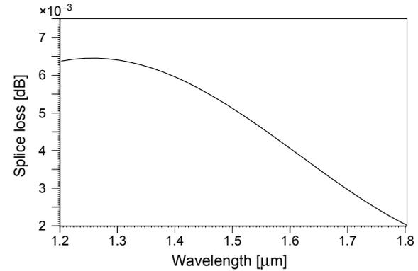
Fig. 12. Variations of splice loss via wavelength of our optimized fiber.
