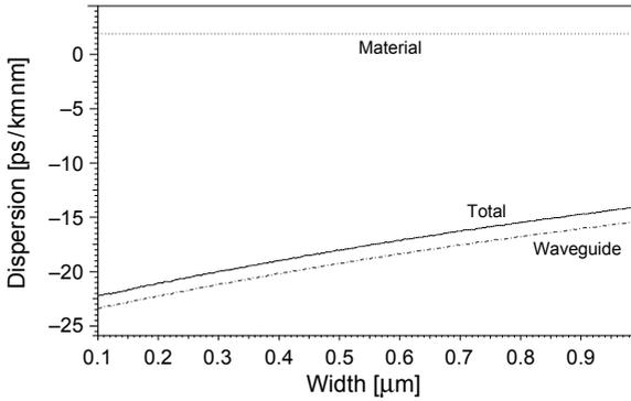
Fig. 21. Dispersion contribution vs. region  $R_4$  width.
