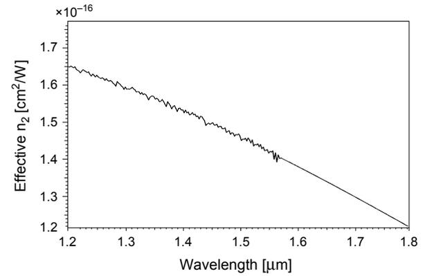
Fig. 10. Variations of  $n_2$  vs. wavelength of our optimized fiber.
